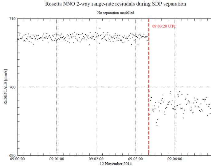
**Figure 5. Range-rate residuals of pass-through around separation**
