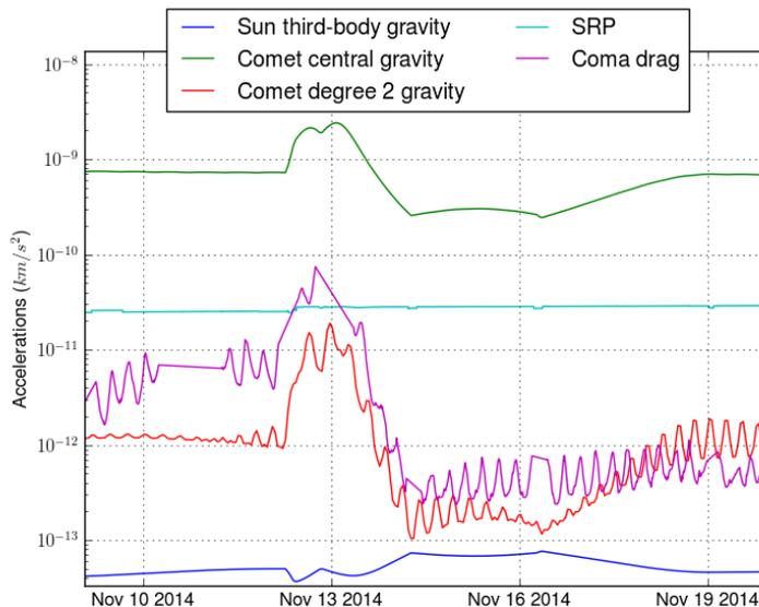
**Figure 6. Rosetta accelerations around landing time**
