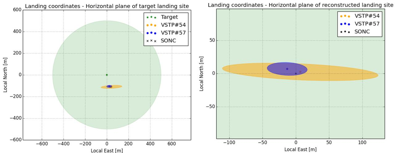
**Figure 12. Reconstructed touch-down point and 3-sigma uncertainty ellipses**
