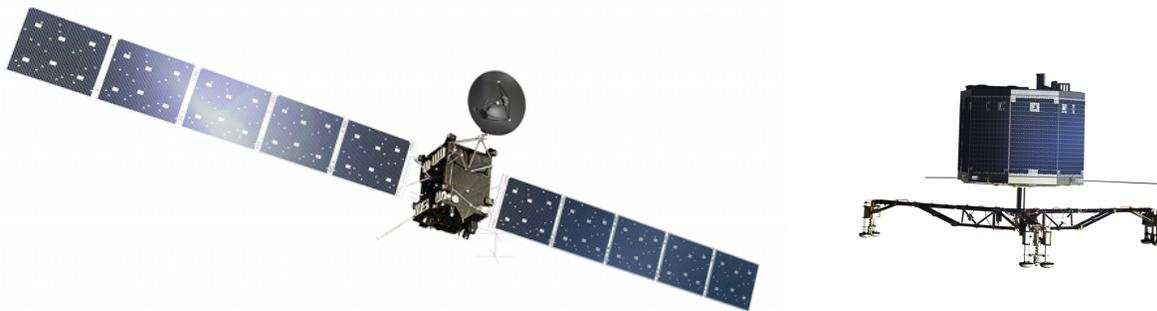
**Figure 1. Rosetta spacecraft (left) and Philae lander (right)**
