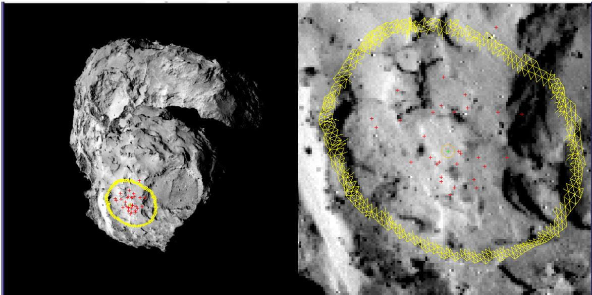
**Figure 3. Landing points of simulated trajectories plotted on top of a NAVCAM image**
