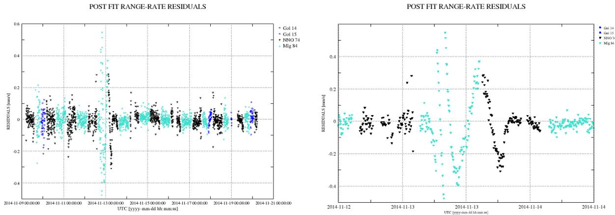
**Figure 7. 2-way range-rate residuals of the final reconstruction (left); zoom around the time of lander delivery (right)**
