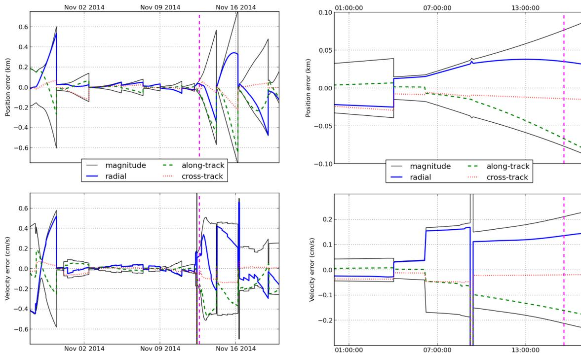
**Figure 9. Orbit prediction errors during Lander Delivery phase (left) and zoom around landing time (right). Landing time is marked in dashed magenta**
