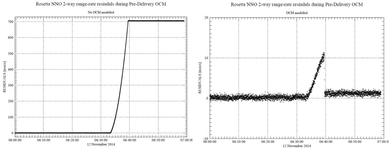
**Figure 4. Range-rate residuals of the pre-delivery manoeuvre pass-through**
