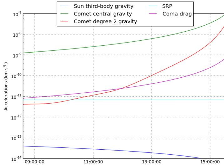
**Figure 10. Philae accelerations during descent**
