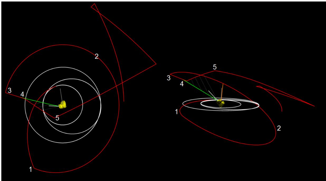
**Figure 2. Lander Delivery trajectory: Rosetta (red), Philae (green). Views from Sun direction (left) and close to the terminator plane (right)**
