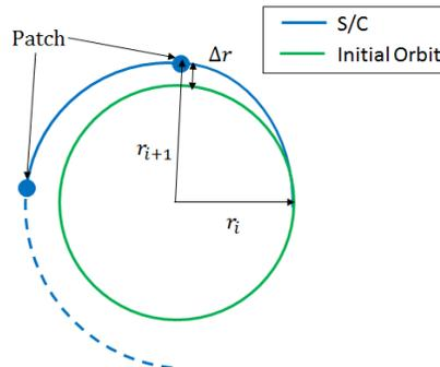
**Figure 2. Patched Conic of Low Thrust Trajectories**
