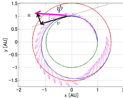
**Figure 1. Circle-to-Circle Transfer with continuous thrust (Earth to Mars)**
