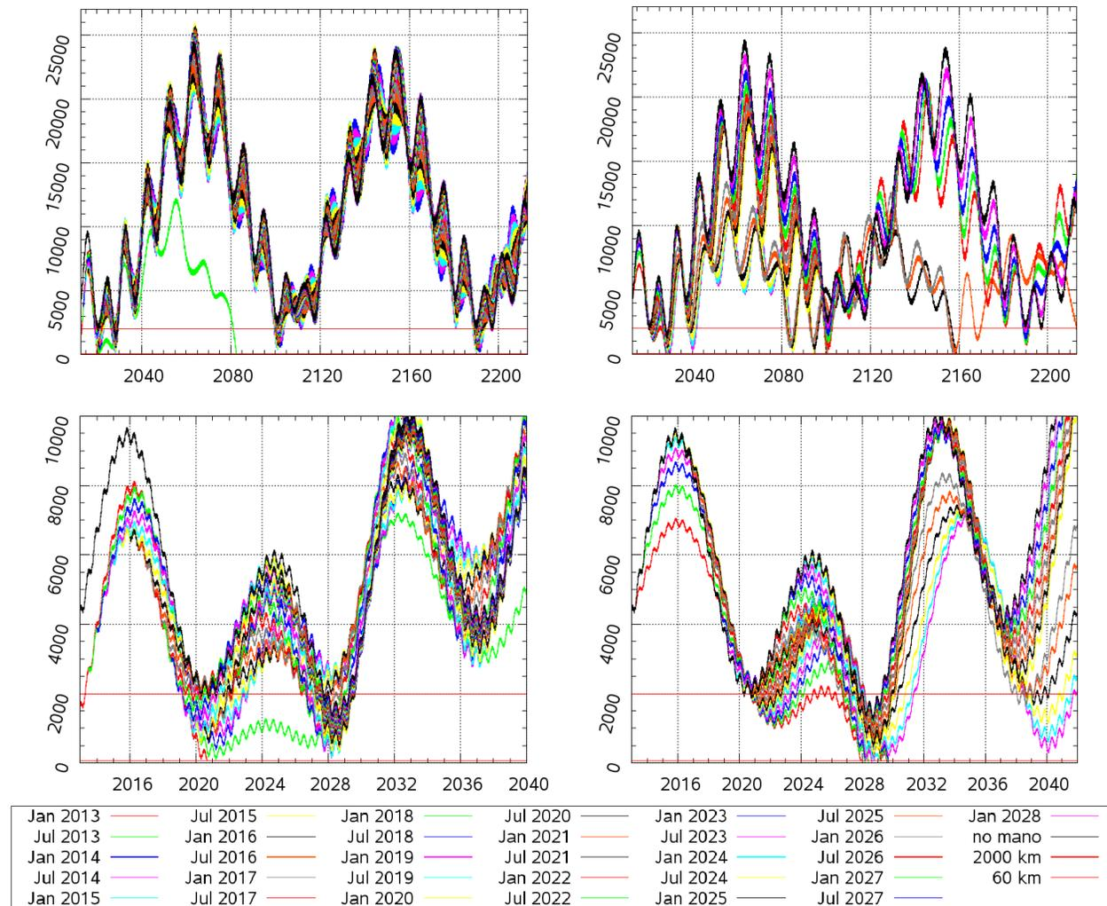
**Figure 6. Perigee altitude evolution for manoeuvres at apogee (left) and perigee (right). Bottom row gives zoom of upper row figures.**
