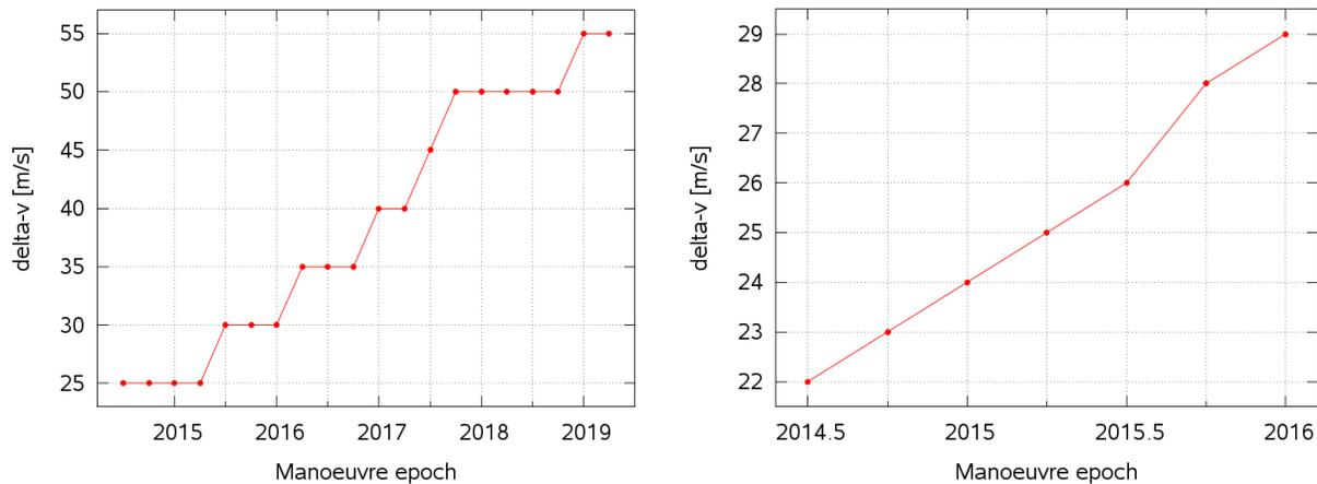
**Figure 7. Minimum delta-v (quarterly screening) needed for re-entry as a function of manoeuvre date. Left: 5 m/s granularity. Right: 1 m/s granularity for early dates**
