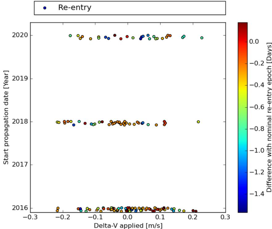
**Figure 10. Re-entry time (as difference w.r.t. nominal time) as function of start epoch and delta-v**
