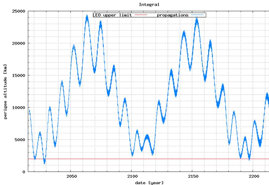
**Figure 2. Evolution of perigee altitude for Integral without manoeuvre. For comparison the upper LEO limit of 2000 km is shown in red.**
