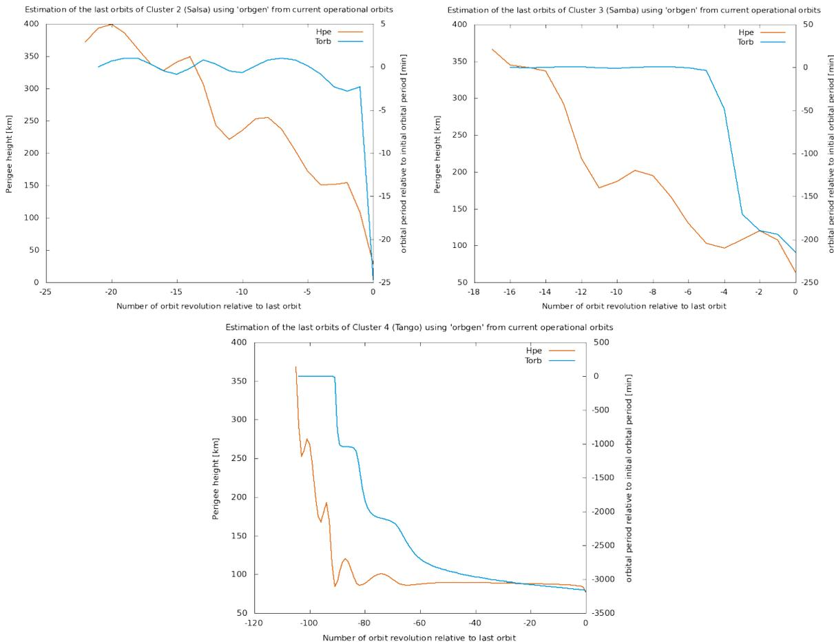
**Figure 9. Perigee altitude [km] and absolute change in orbit revolution time [minutes] for the last perigee passages till re-entry for Cluster-2 (top left), Cluster-3 (top right), Cluster-4 (bottom) based on an operational orbit of epoch 2014**
