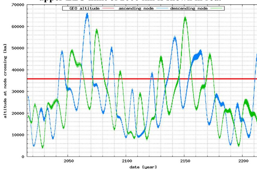
**Figure 3. Altitude at node crossings for Integral without manoeuvre. For comparison the upper protected GEO altitude range shown in red.**
