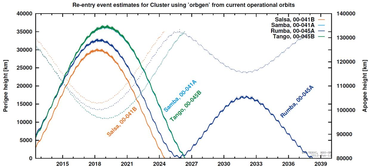
**Figure 4: Evolution of perigee and apogee height for the 4 Cluster spacecraft without manoeuvre.**
