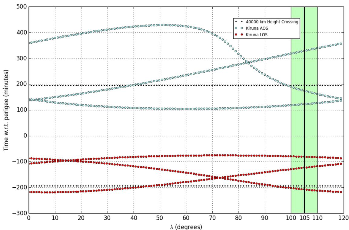
**Figure 3: Kiruna ground station visibility in the three revolutions as a function of  $\lambda$ . The green region represents the target of  $\lambda = 105$  degrees with a 5 degree band.**
