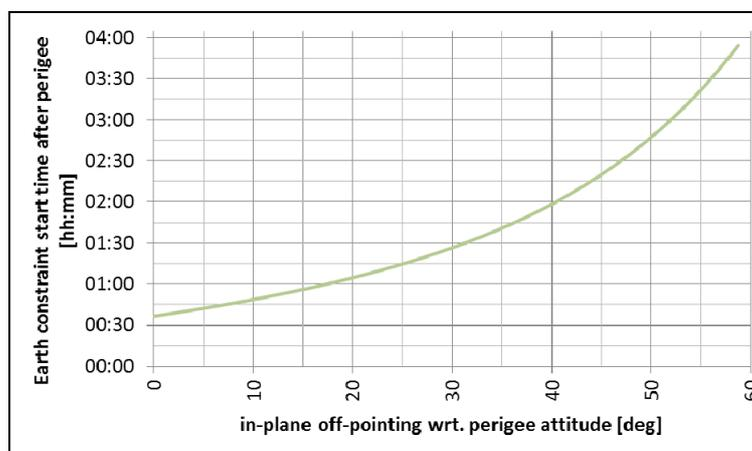
**Figure 5: Earth constraint start time versus in-plane off-pointed attitude angle**
