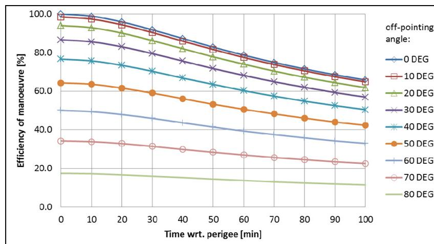
Figure 4: Efficiency of an impulsive manoeuvre with non-optimal attitudes and timing
