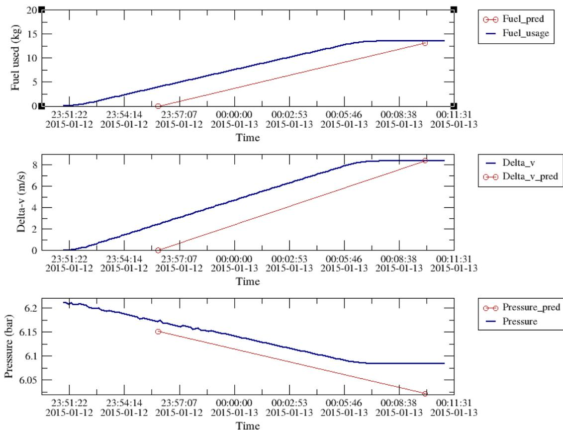
**Figure 9: Thruster monitoring plot from manoeuvre 1; predicted values are in red, measured in blue**
