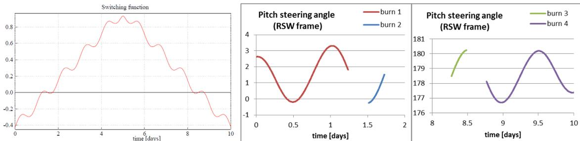
**Figure 10. Switching and pitch steering angle during a GEO relocation.**
