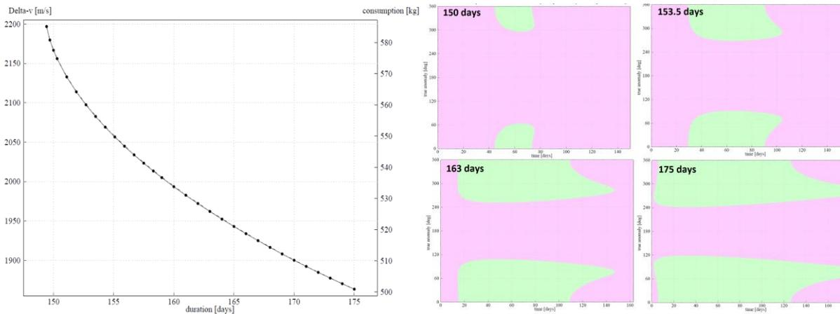
**Figure 8. Left: delta-v and consumption as function of transfer duration. Right: optimum (magenta)/ off (green) periods for 4 selected durations.**
