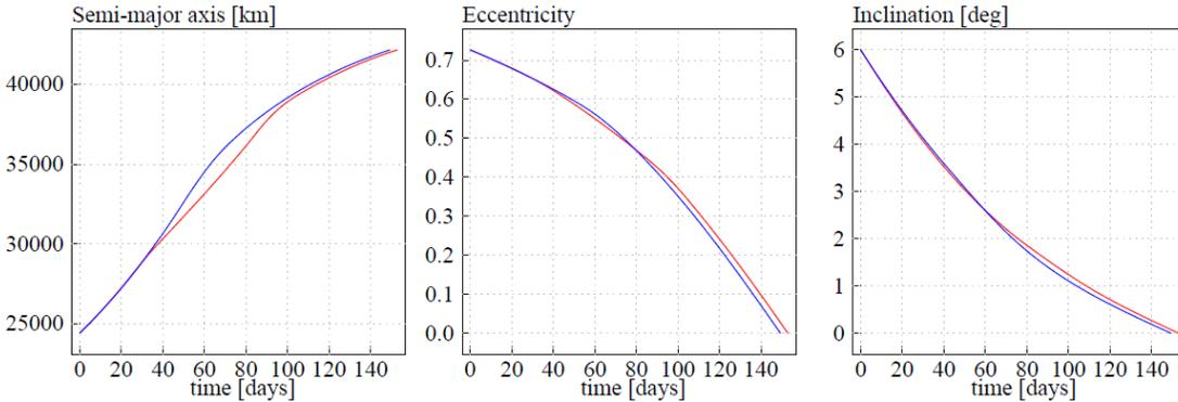
**Figure 7. Time evolution of  $a$ ,  $e$ ,  $i$  for min duration (blue) and min fuel with 153 days (red).**
