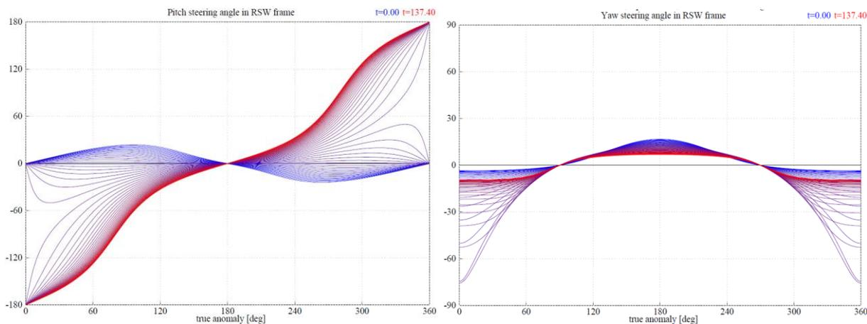
**Figure 1. Left: in-plane (pitch) steering angle. Right: out-of-plane (yaw) steering angle for case 1. Blue is  $t=0$ , red is  $t=137$ .**
