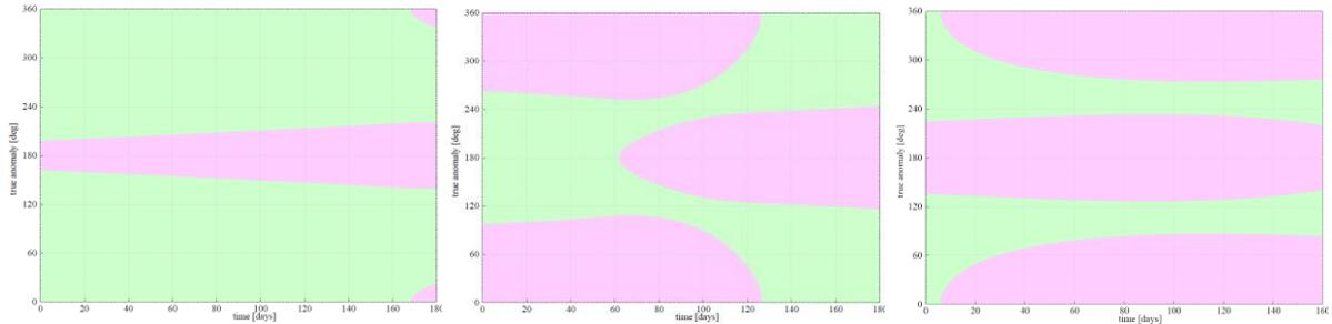
**Figure 3. Optimum on (magenta) / off (green) periods for the solutions of Case 5 = GTO→GEO, Case 6 = MEO→GEO and Case 7 = SSTO→GEO (left to right)**
