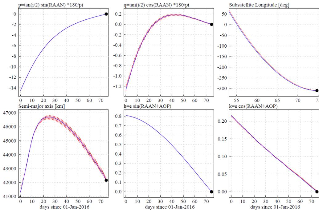
**Figure 5. Time evolution of equinoctial elements for averaged (blue) and non-averaged (red) method. Note that only the last 20 days are displayed for the subsatellite longitude.**
