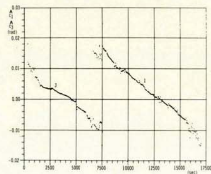
Fig. 35 Estimated earth chord delays of first and third earth sensor (real free-drift 4, case 2)
