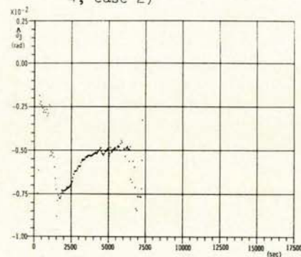
Fig. 36 Estimated delay of midscan rotation angle measurements of third earth sensor (real free-drift 4, case 2)
