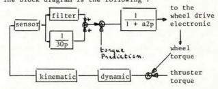
A torque prediction is incorporated in the loop in order to minimise the pitch transient response due to the dynamics of the loop.
