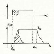
$F_{o}$  : nominal thrust  $d_{R}$ ,  $d_{C}$  : pure delay /// : short pulse
