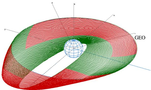
**Fig. 2: Inclined initial orbit (Super-GTO 55 000 km and 28.5°) to GEO with Apogee and Perigee-centred thrust arcs.** The total number of orbits is 178.
