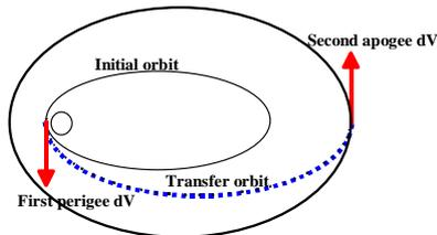
**Fig. 4: First phase of a continuous transfer: Equivalence with the classical Hohmann impulse transfer.**
