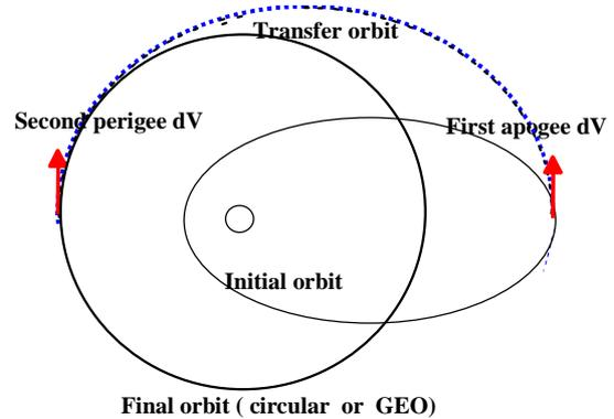
**Fig. 5: Second phase of a continuous transfer: Equivalence with the classical Bi-elliptic impulse transfer.**
