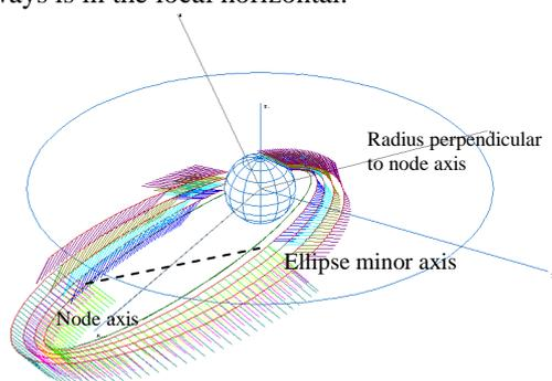
**Fig. 4 Orbit Transfer from inclined orbit, First Phase** (2 transition zones: one at the ellipse minor axis for Perigee and Apogee altitude increase, one at the radius perpendicular to the orbital node for the inclination change)
