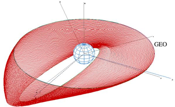
**Fig. 3: Continuous Orbit Transfer from an Inclined initial orbit (Super-GTO 60 000 km and 28.5°) to GEO.** The total number of orbits is only 91.
