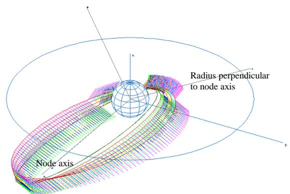
**Fig. 5 Orbit Transfer Second Phase (in-plane component inertial)** (1 transition zone, due to inclination change, at the radius perpendicular to the orbital node)
