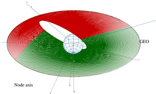
**Fig. 1: Inclined initial orbit (Sub-GTO 28.5°) to GEO with Apogee-centred thrust arcs.** Note that the effects of the large thrust arcs with a large increase of the perigee altitude, and a slight increase of apogee altitude. The total number of orbits is 295.
