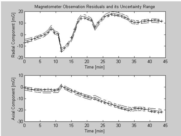
**Figure 2: Residuals of SCD-1 at 30<sup>th</sup> iteration; Orbit # 5268-5271, real data**
