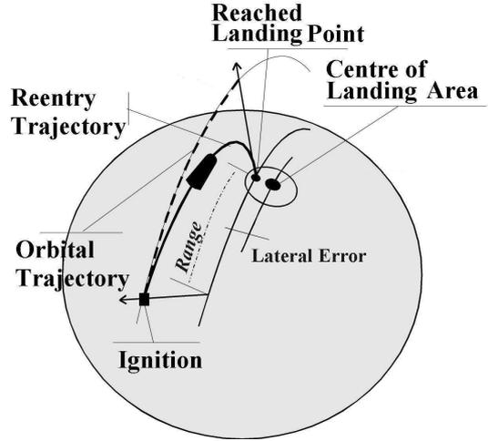
Figure 3 - Illustration of lateral error, reentry trajectory and landing area.
