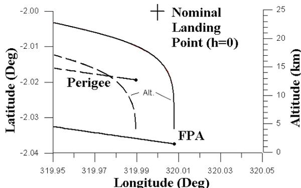
**Figure 6 - Details of the trajectories of vehicle below 25 km for criteria FPA and *Perigee*.**
