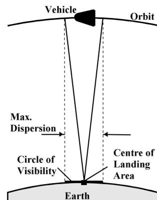
Figure 3 - Projection of Visibility Cone.
