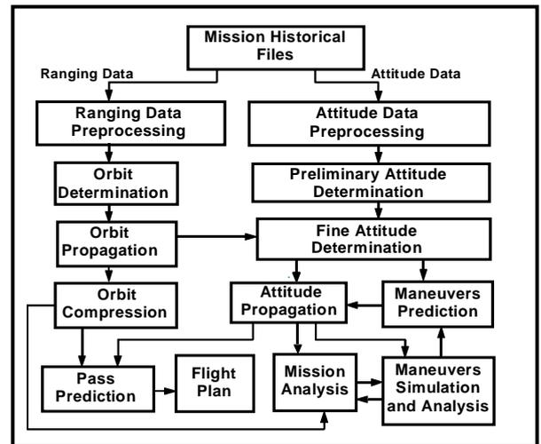
Fig. 1 - Flight Dynamics System
