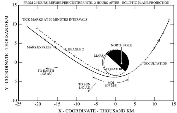
Fig. 9. Mars Express Mars orbit insertion (MOI)
