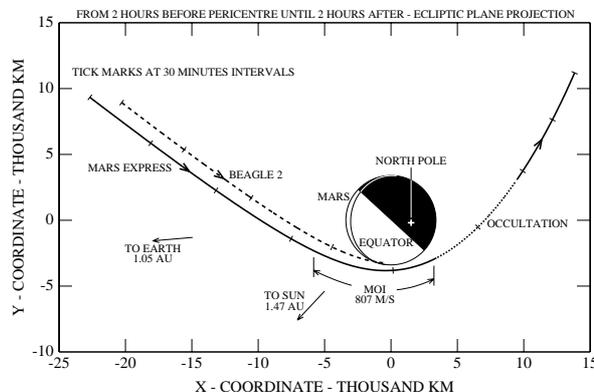
Fig. 9. Mars Express Mars orbit insertion (MOI)
