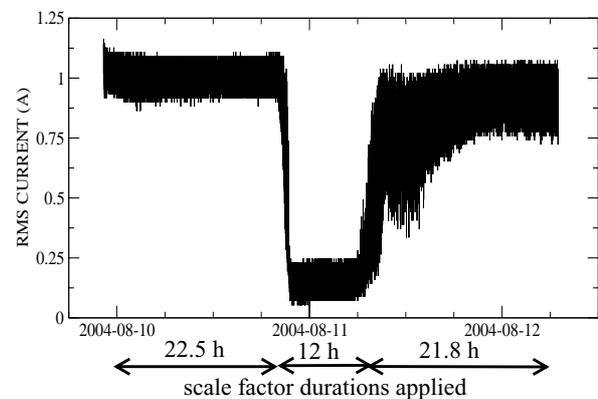
Fig. 2. Rms anode current and scale factor splitting.
