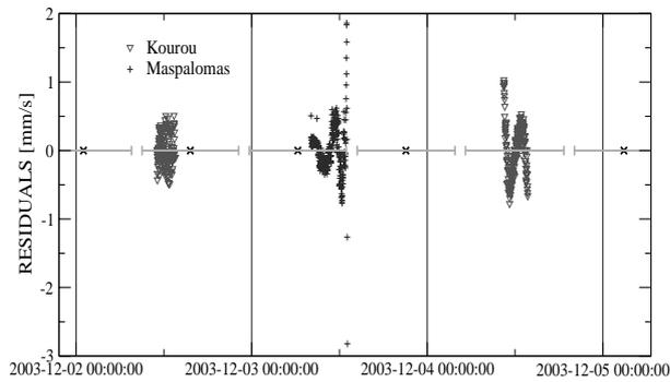
Fig. 3. Doppler residuals of an early orbit determination.
