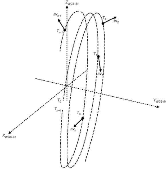
Fig. 3. Target trajectory (167 revolutions). Maneuvers take place at times  $T_i=1, 2, \dots, n$ .
