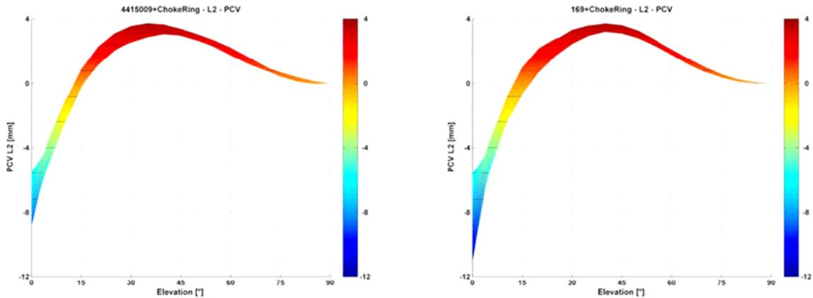
**Fig. 10** L2 phase center variations for two test units of a Sensor Systems S67-1575-14 (*left*) and -141 antenna (*right*). The width of the both graphs represents the variation of the phase center for different azimuth angles.
