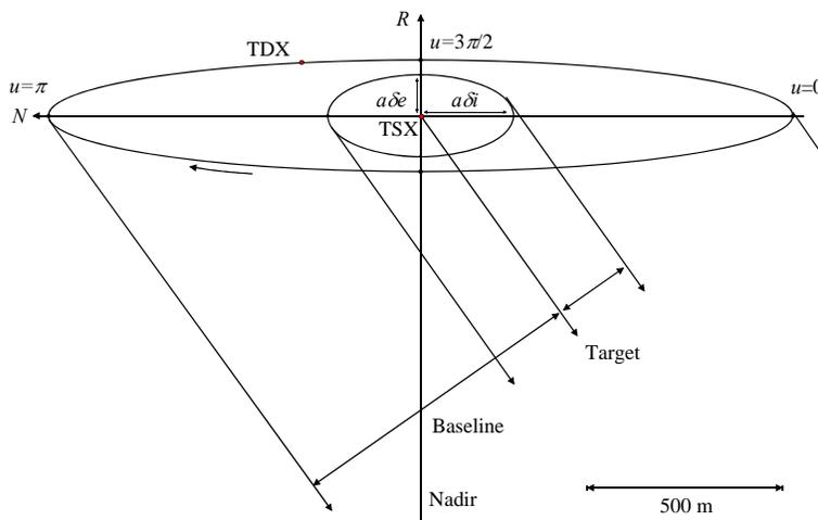
**Fig. 2** Relative motion of TDX with respect to TSX (as seen in flight direction) and projected baseline for different eccentricities ( $a\delta e=200\dots300\text{m}$ ) and relative inclinations ( $a\delta i=500\dots2000\text{m}$ ).
