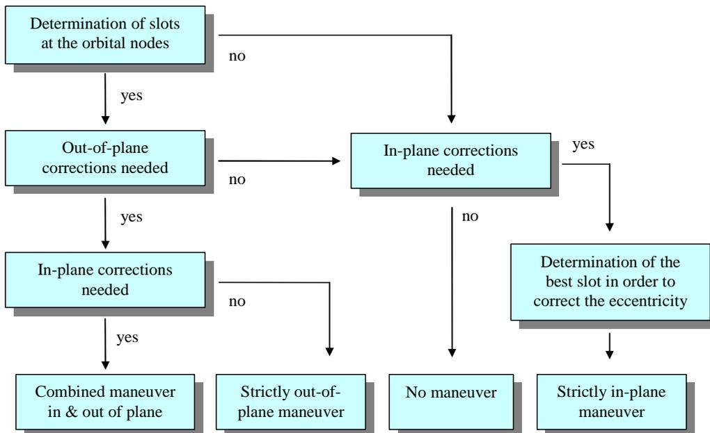
**Figure 12. Slot selection algorithm**
