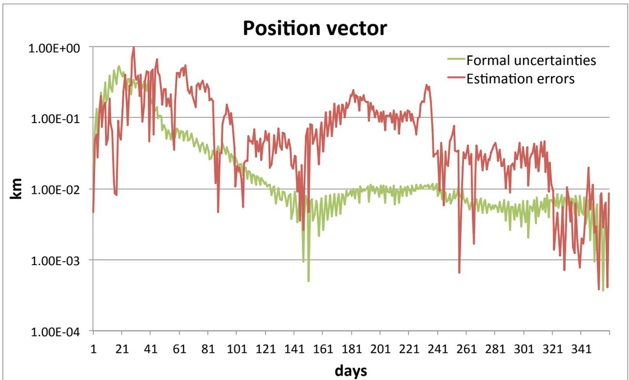
**Figure 6. Estimation errors and formal uncertainties in position for the batch-sequential filter.**
