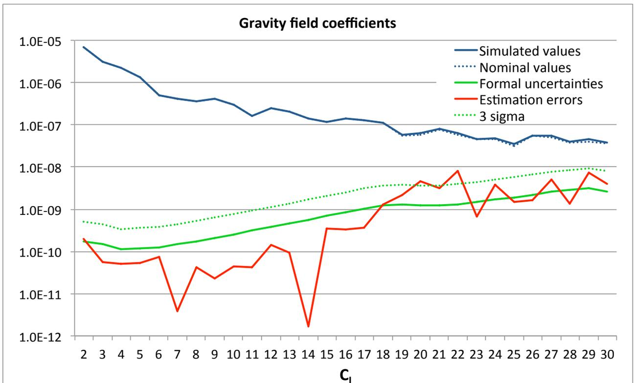
**Figure 9. Final estimate of the gravity field coefficients, after multiarc step.**
