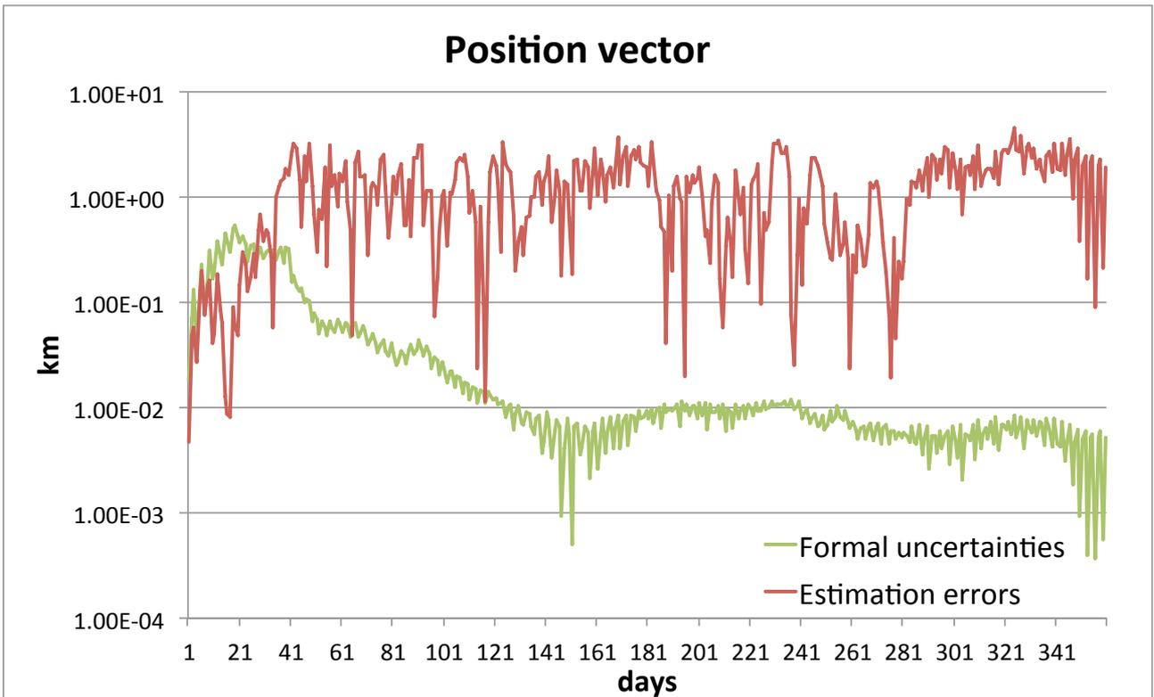
**Figure 4. Real errors and formal uncertainties in the estimation of the spatial components of the state vector, for a classical batch estimation. The y-axis shows the norm of the position error vector.**
