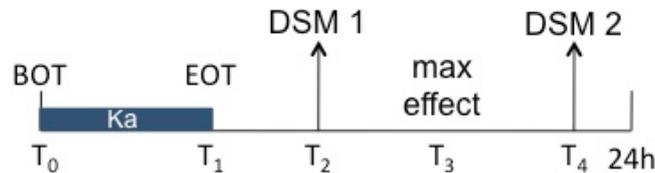
**Figure 1 - Tracking period and wheel desaturation maneuvers (DSM)**
