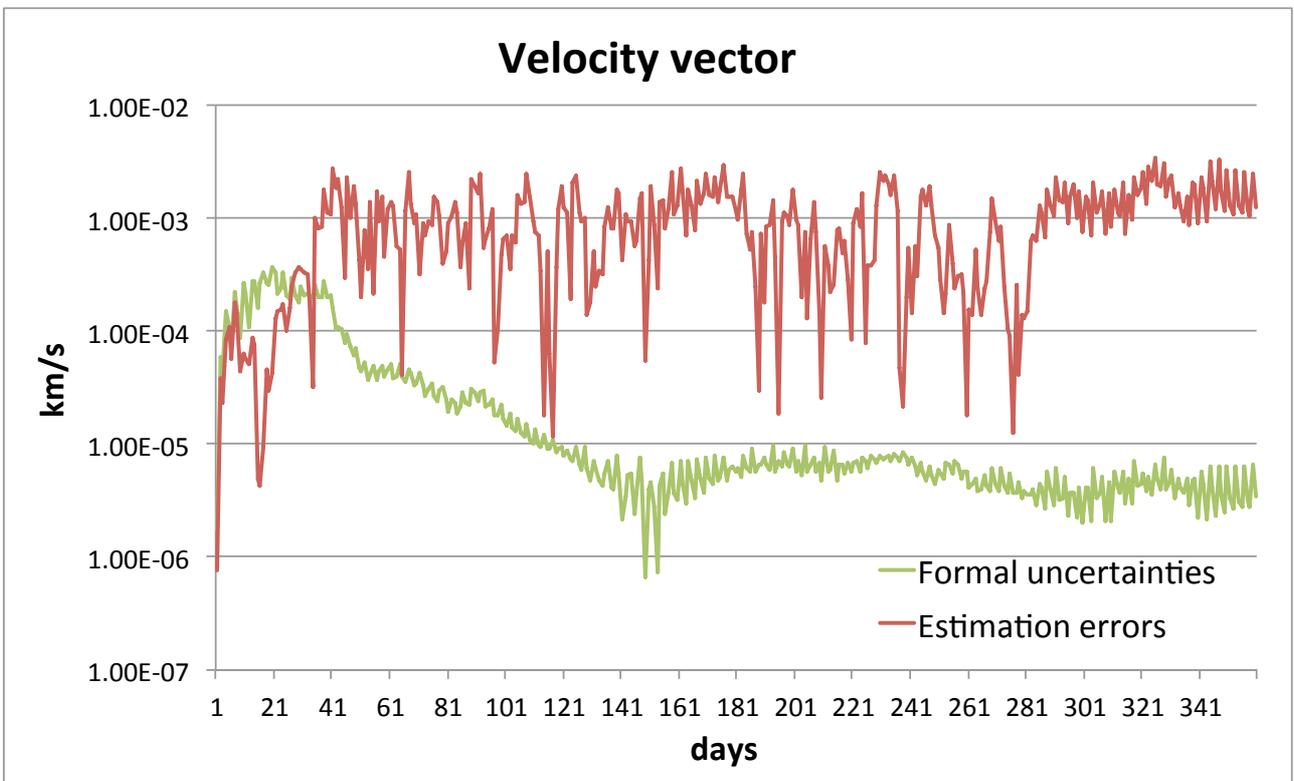
**Figure 5. Real errors and formal uncertainties in velocity vector estimation by means of classical batch estimation.**
