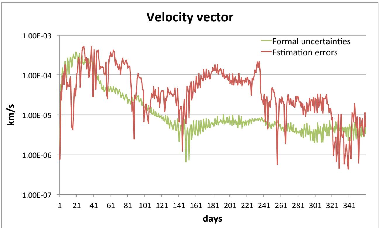
**Figure 7. Estimation errors and formal uncertainties in velocity for the batch-sequential filter.**
