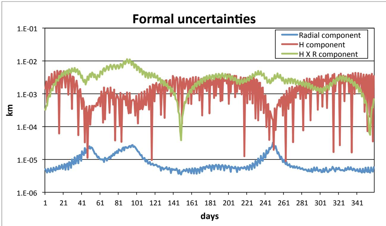
**Figure 10. Uncertainties in position after final orbit reconstruction (in the orbital frame).**
