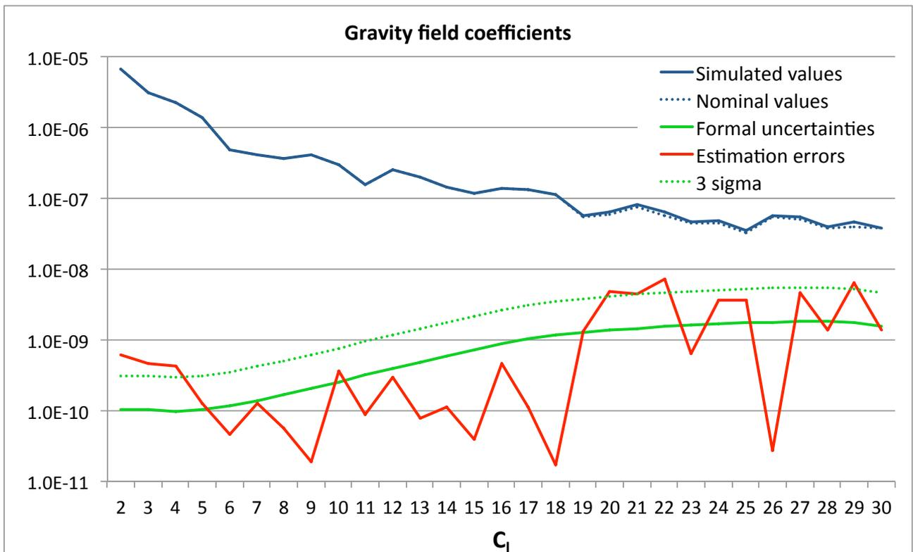
**Figure 8. Estimation errors and formal uncertainties of gravity harmonics coefficients, from the batch-sequential filter.**
