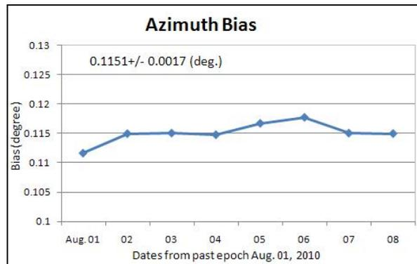
**Figure 1. COMS satellite azimuth bias estimation by orbit determination**
