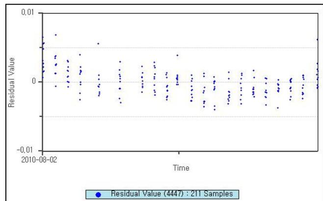
**Figure 3. Azimuth and elevation residuals of Daejeon station for the date of Aug. 2, 2010**
