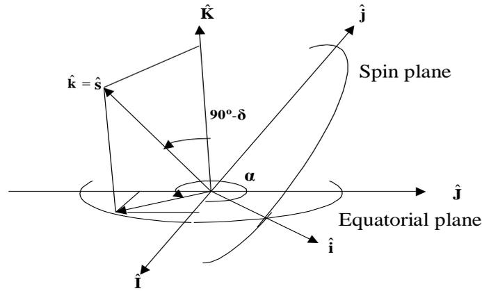
**Figure 1** - Orientation of the spin axis ( $\hat{s}$ ): Equatorial System ( $\hat{I}, \hat{J}, \hat{K}$ ), satellite body frame reference system ( $\hat{i}, \hat{j}, \hat{k}$ ), right ascension ( $\alpha$ ) and declination ( $\delta$ ) of the spin axis.
