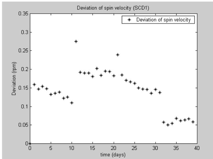
**Figure 5 - Temporal behavior of the difference between the real and computed value of the spin velocity, with daily updated data.**
