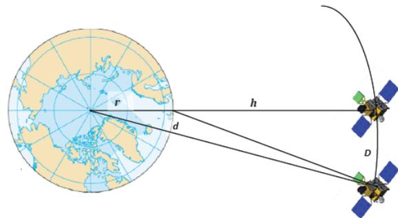
**Figure 2: Attitude estimated in Earth-fixed frame: parallax effect of position error D on geolocation**
