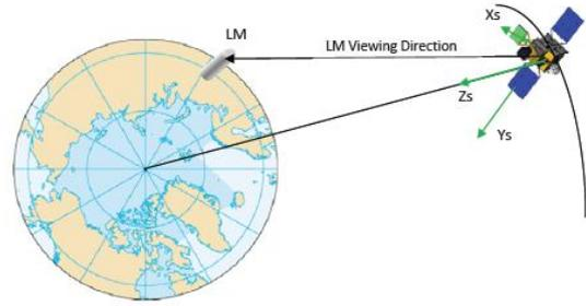
**Figure 4: LM view direction in satellite reference frame**
