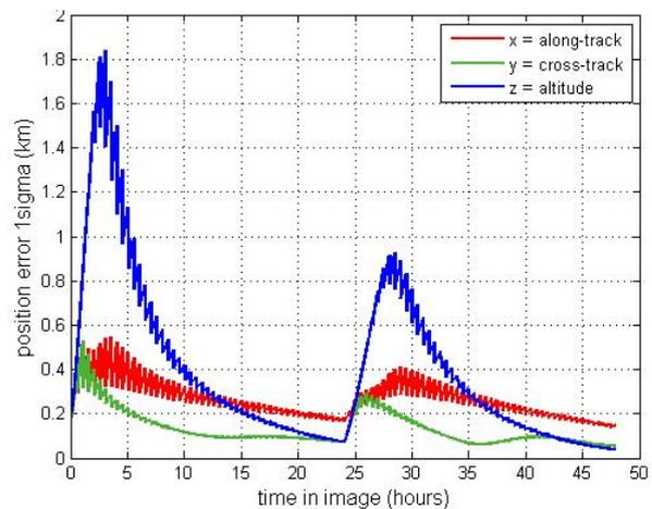
**Figure 9: Transient time with no ranging; LM every 30 min**
