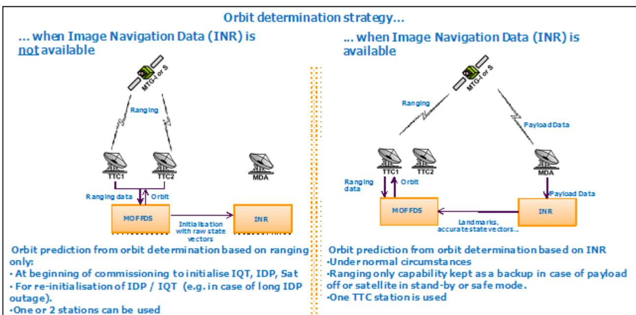
**Figure 13: Orbit Determination with & without INR**
