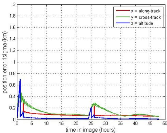
**Figure 8: Transient time with 1 station ranging; LM every 30 min**
