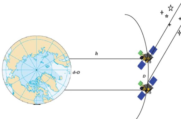
**Figure 1: Attitude estimated in inertial frame: direct effect of position D error on geolocation**
