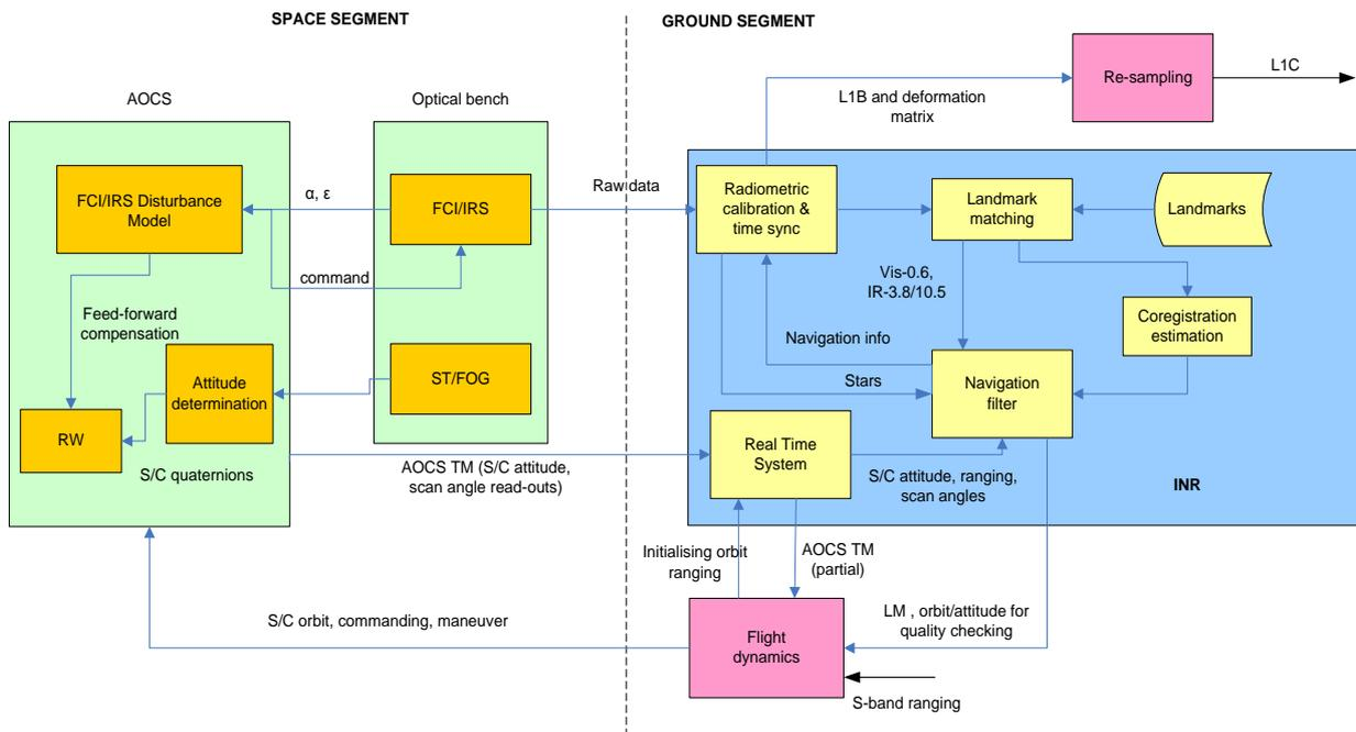
**Figure 10: INR and FD system architecture design**
