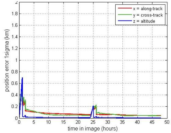
**Figure 7: Transient time with dual ranging every hour and LM every 30 minutes**
