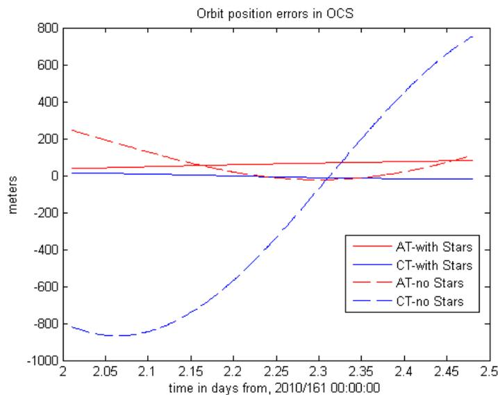
**Figure 12: Cross-track and Along-track errors with and without stars**
