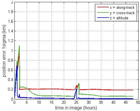
**Figure 6: Transient time with dual ranging every hour**
