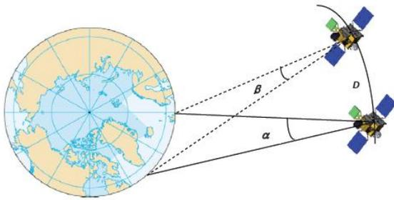
**Figure 3: Parallax effect on differential LM view angle**
