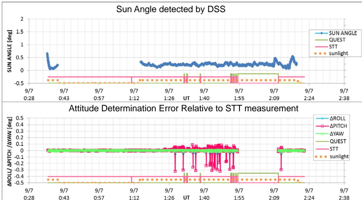
**Figure 13. Attitude Determination Error After Operation for Improvement**
