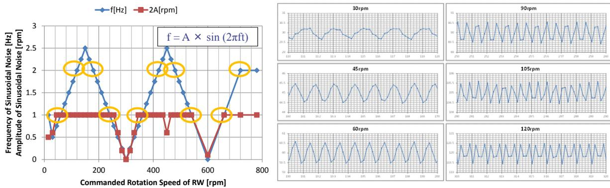
**Figure 19. Sinusoidal Noise on the RW Rotation Speed**
