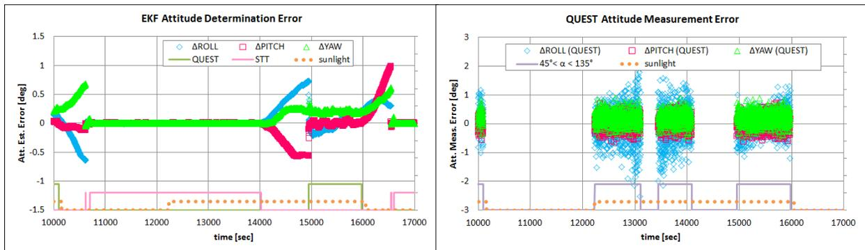
**Figure 9. Attitude Determination Error in One Orbital Period**
