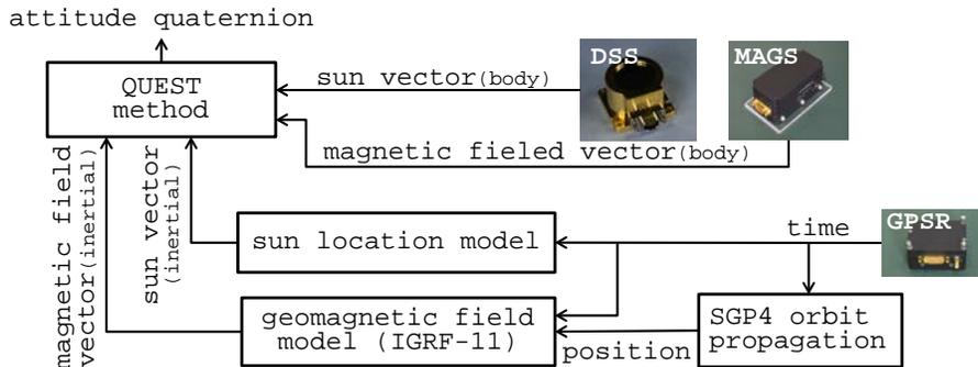
**Figure 5. Schematic Diagram of the QUEST attitude measurement**
