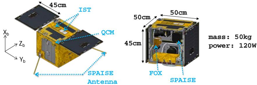
**Figure 1. Small Demonstration Satellite 4 (SDS-4)**
