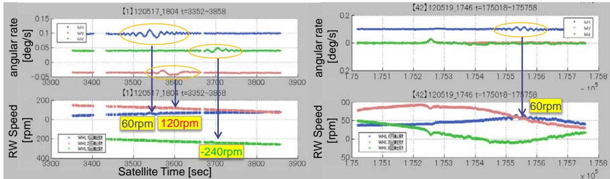
**Figure 18. Oscillatory Response in Satellite’s angular rate and RW Rotation Speed**
