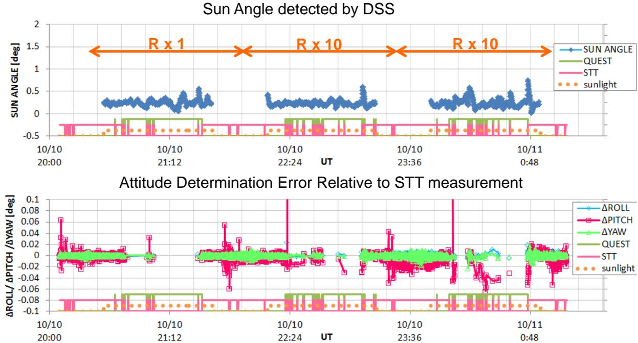
Figure 14. Attitude Determination Error at R = 1R, 10R, and 100R
