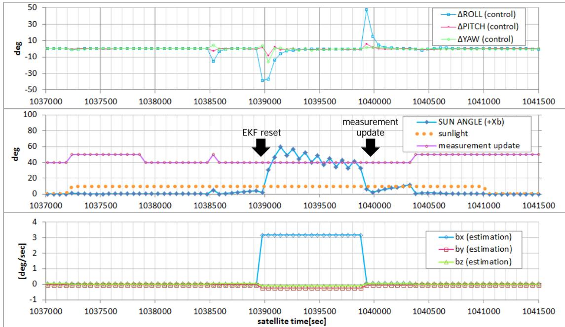
**Figure 16. Unexpected Loss of Attitude due to the EKF Reset**
