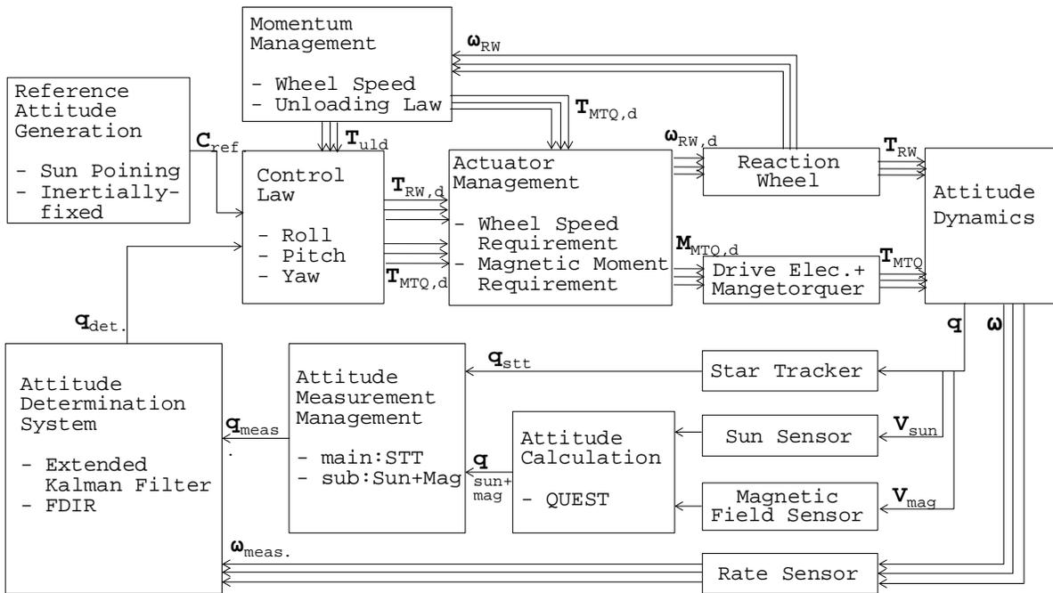
Figure 3. ACS closed-loop block diagram
