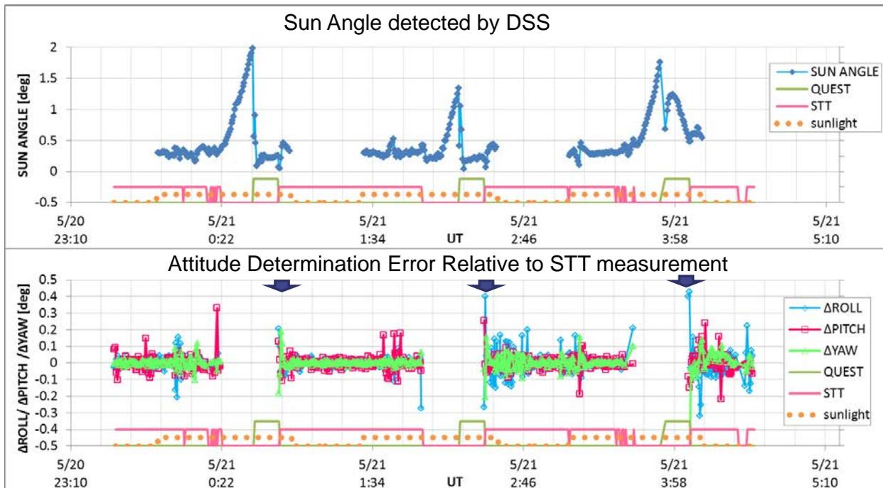
**Figure 12. Attitude Determination Error in the Early Operation (3 orbital periods)**
