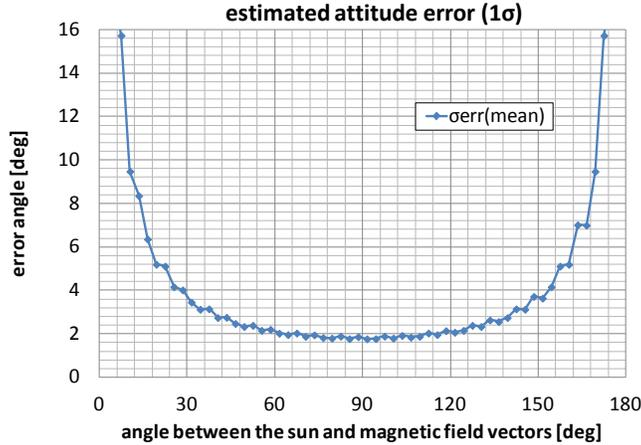
**Figure 6. Estimated Attitude Error ( $1\sigma$ ) in the QUEST method**
