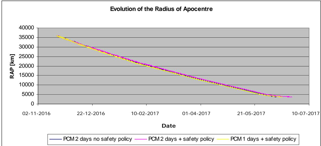
To consider potential failures of maneuvers increases the duration of the aerobraking by several days (Fig. 1).
