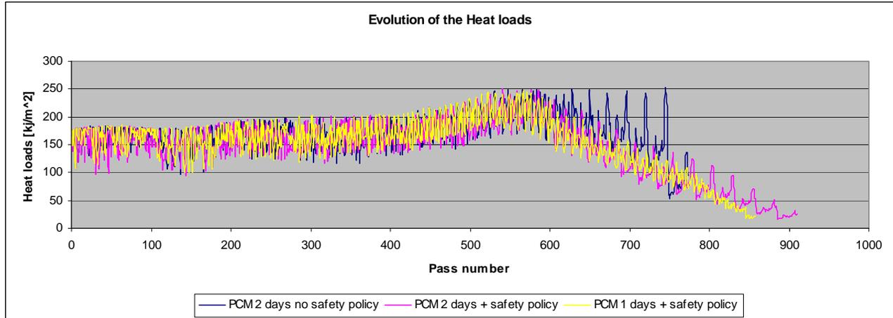
The walk-out phase starts approximately at the pass 600. The maximum heat load is only achieved in the simulation without safety policy. This happens because in the other cases the maximum head loads are found on the 48 extra propagated hours,
