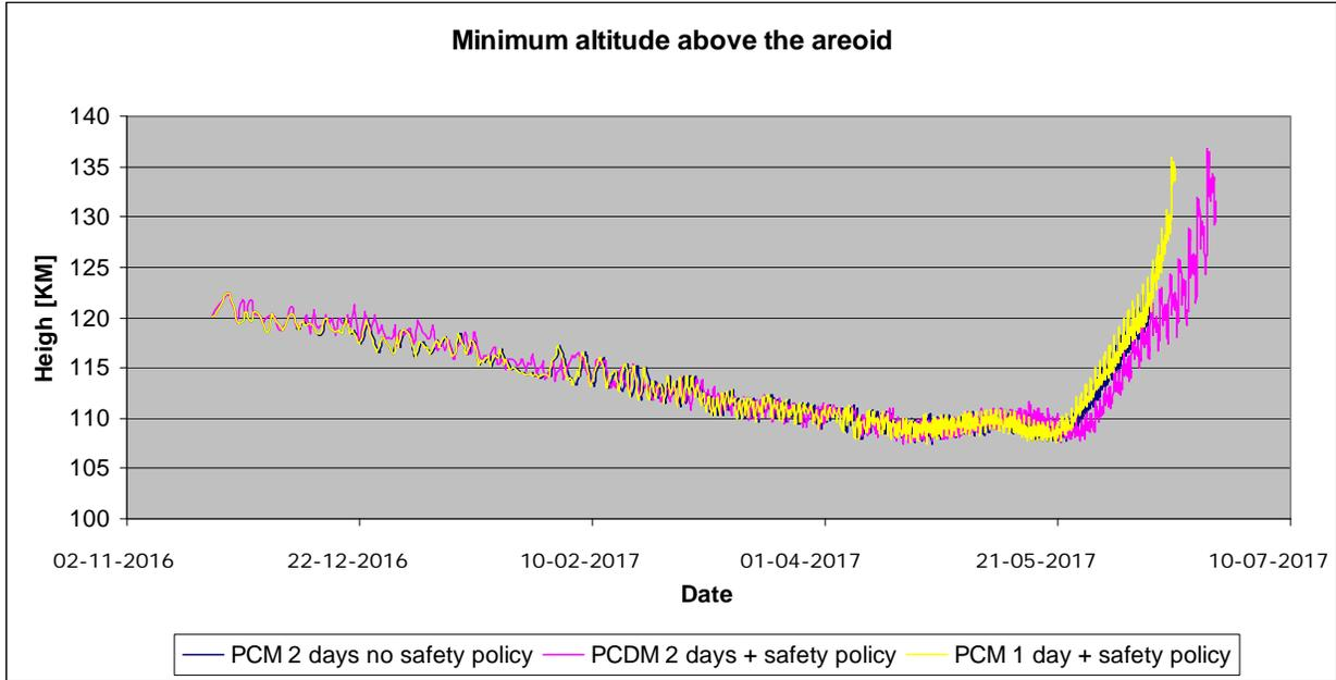
As the spacecraft velocity is decreasing, the pericenter shall be reduced in order to obtain higher density and keep the maximum value of aerodynamic constraints constant, Fig. 2. The active constraint is the peak heat flux and the dynamic pressure.
