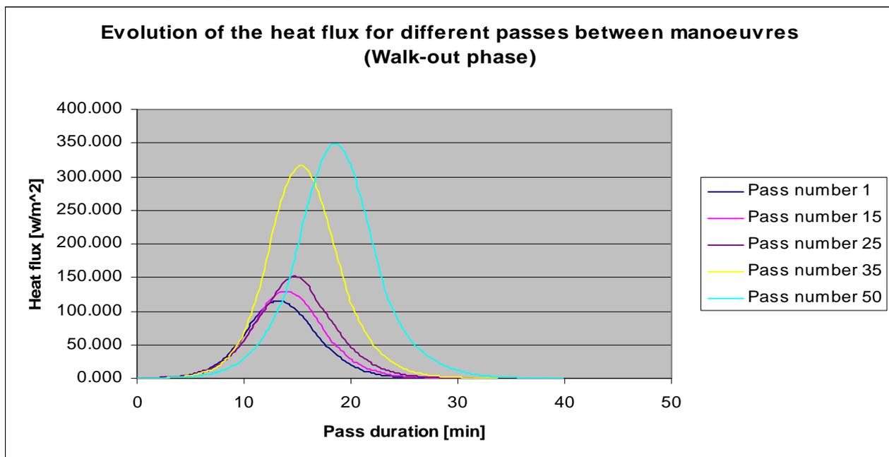
**Figure 8. Heat loads after different maneuvers**
