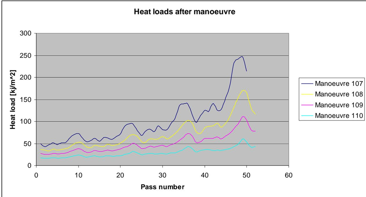
Figure 7 plots the evolution of the heat flux after the maneuver 107 (from a total of 110). The peak values increase each pass, so the active constraint is at the pass number 49. However, if there is no maneuver failure, the pass number 49 will never exist, because the next PCM (maneuver 108) will be performed after the pass 25.
