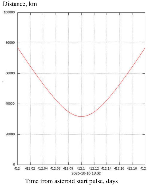
**Figure 7. Distance from the 2011 UK10 asteroid to the Earth center in the region of perigee during gravity assist maneuver.**
