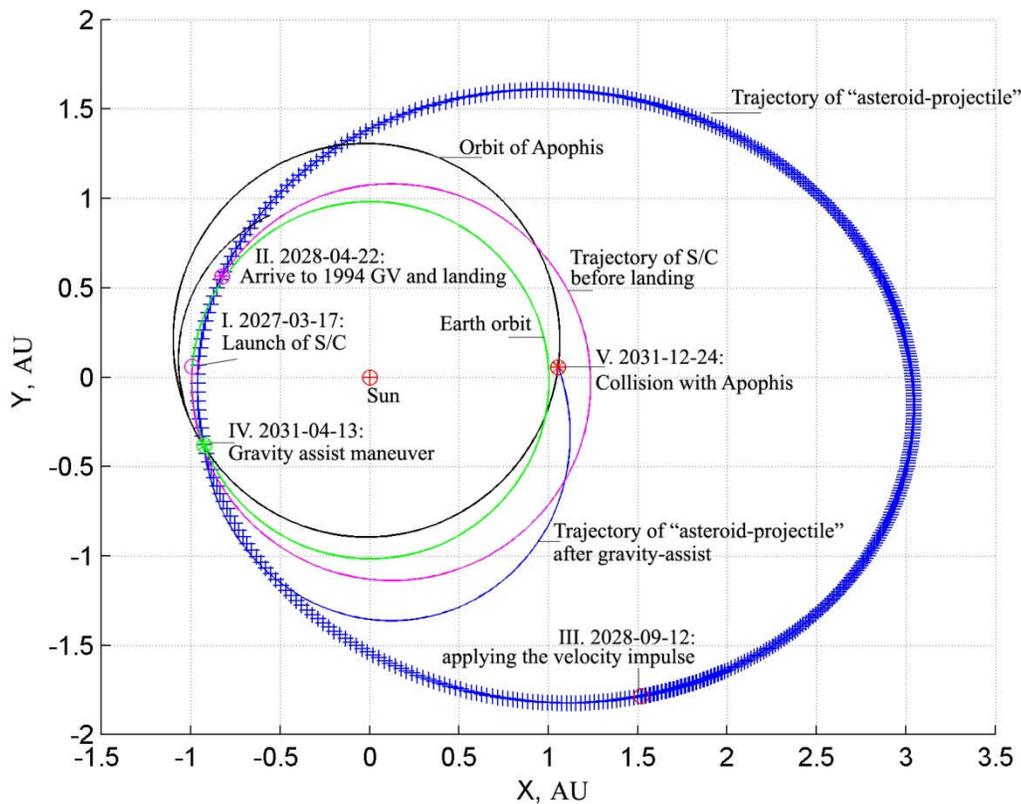
**Figure 9. Trajectories of the Earth, Apophis, asteroid-projectile 1994 GV and spacecraft transfer trajectory from the Earth to 1994 GV.**
