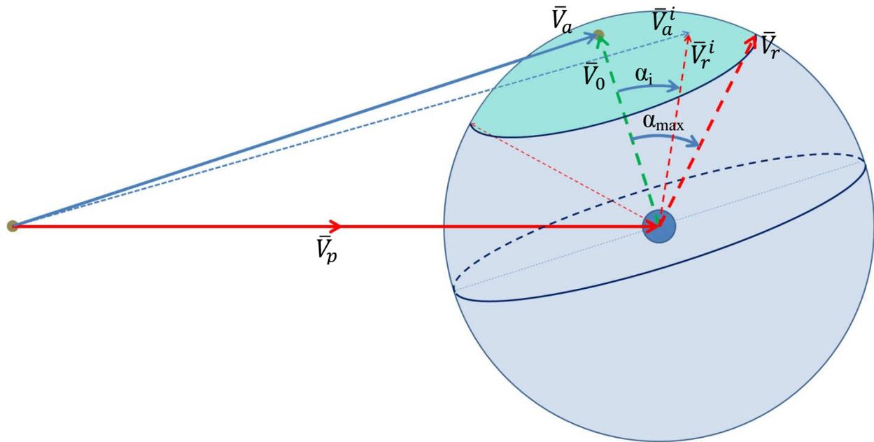
**Figure 2. Geometry of gravity assist maneuver in coordinate system connected with Sun**
