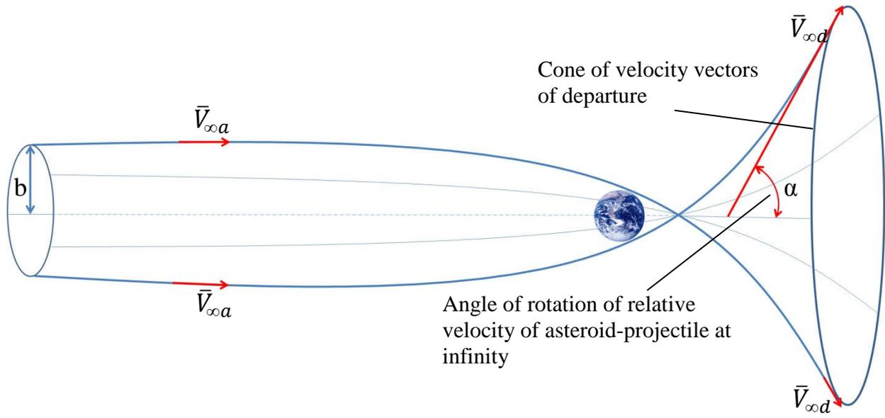
**Figure 1. Cylinder of possible vectors of relative velocities at arrival and resulted after fly-by cone of velocity vectors of departure are imaged**
