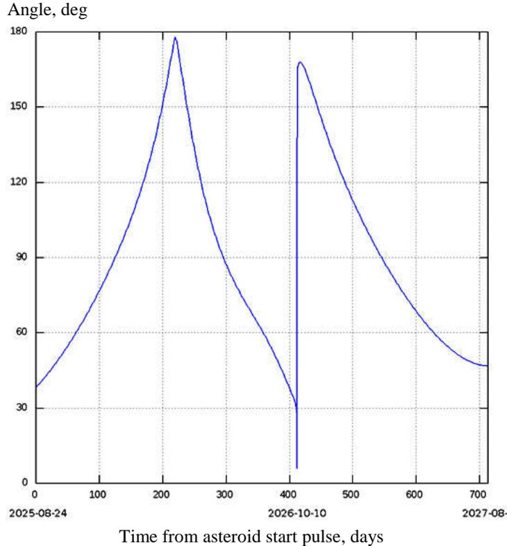
**Figure 8. Earth-asteroid-Sun angle during the mission after 2011 UK10 start to the Earth vicinity for gravity assist maneuver.**
