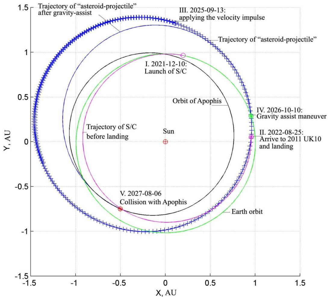
**Figure 5. Trajectories of Earth, Apophis, asteroid-projectile 2011 UK and spacecraft transfer trajectory from Earth to 2011 UK**
