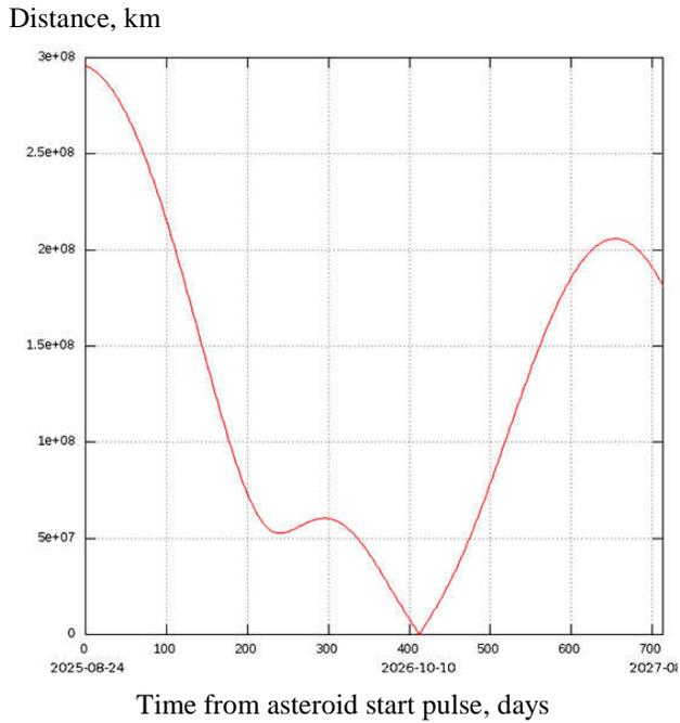
**Figure 6. Distance from the 2011 UK10 asteroid to the Earth center for the time interval from asteroid start pulse to the impact with Apophis.**
