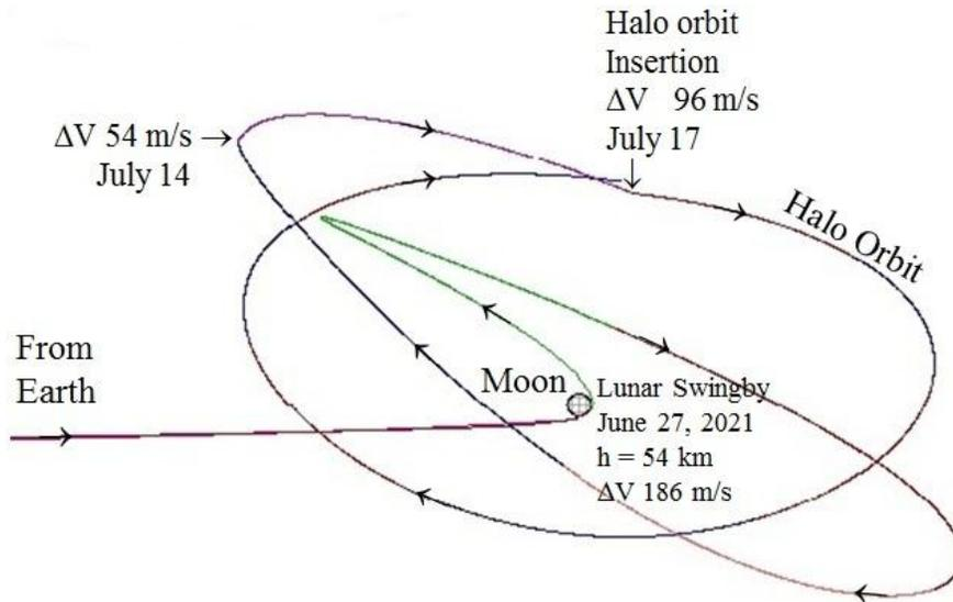
**Figure 12. View from the Earth of the trajectory shown in Fig. 11. The horizontal direction passing through the Moon is the lunar orbit plane, while the vertical direction is perpendicular to the lunar orbit plane.**
