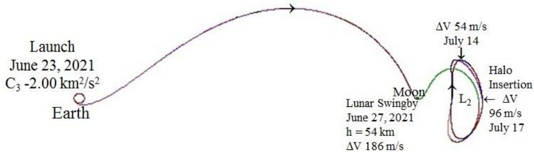
**Figure 9. Indirect transfer from a KSC launch to an Earth-Moon L2 halo orbit using a realistic force model. Rotating lunar orbit plane view, fixed horizontal Earth-Moon line.**
