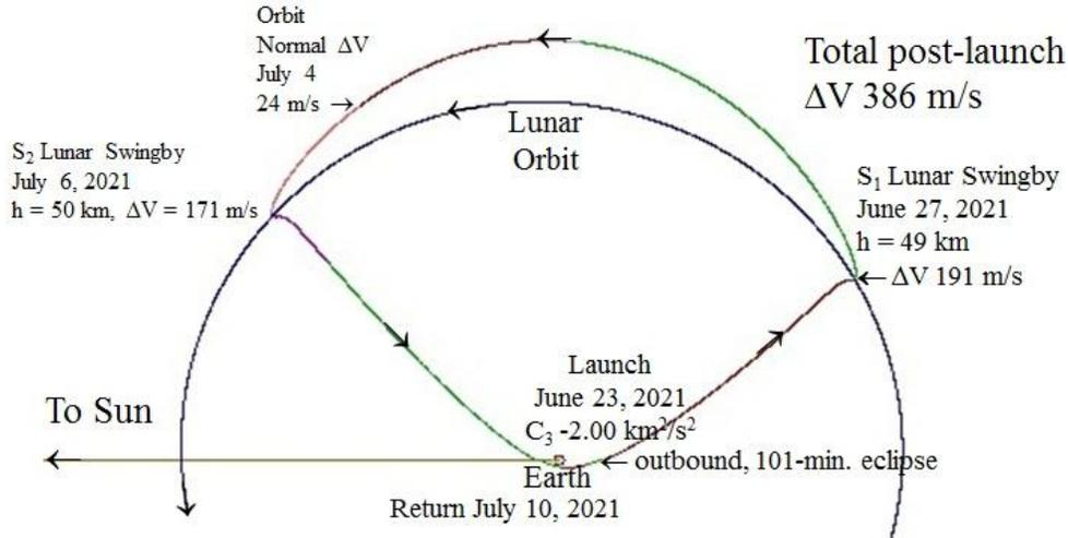
**Figure 5. The trajectory shown in Fig. 4 in a rotating ecliptic plane view with a fixed horizontal Sun-Earth line.**
