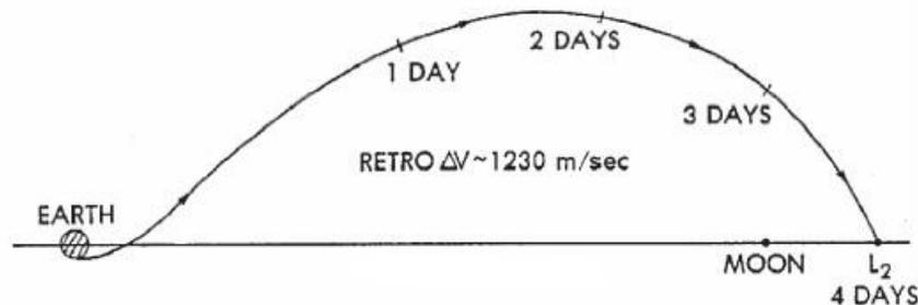
**Figure 1. Direct transfer from a low-Earth parking orbit to the Earth-Moon L2 point. Rotating lunar orbit plane view with a fixed horizontal Earth-Moon line [8, 10].**
