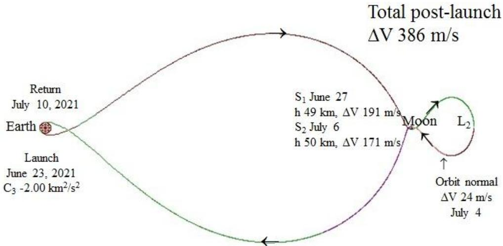
**Figure 4. Indirect transfer from a KSC launch to near the Earth-Moon L2 point and return using a realistic force model. This is a rotating lunar orbit plane view with a fixed horizontal Earth-Moon line.**
