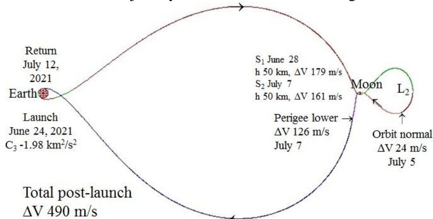
**Figure 8. A 17-day trajectory like that shown in Fig. 4 but with launch a day later. Rotating ecliptic plane view with fixed horizontal Sun-Earth line.**
