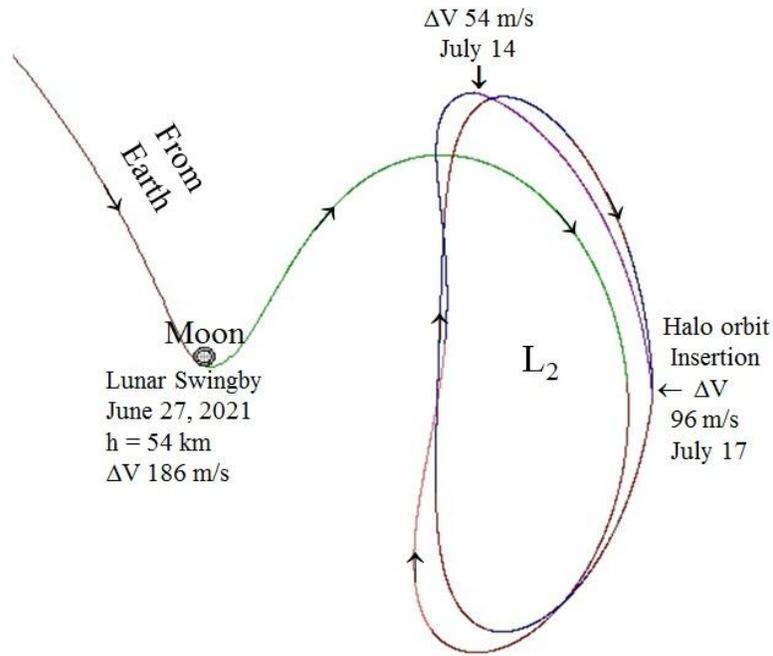
**Figure 11. An expanded view near the Moon of the trajectory shown in Fig. 9, also in a rotating lunar orbit plane view with a fixed horizontal Earth-Moon line.**
