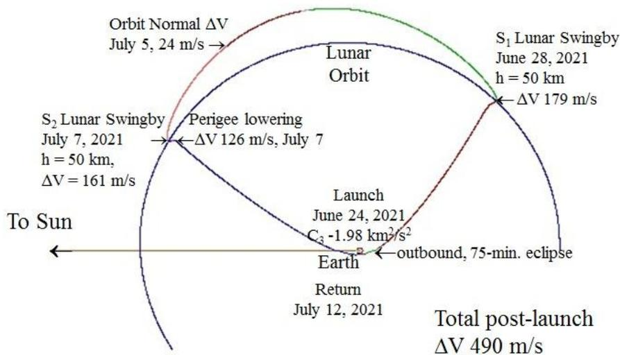
**Figure 7. A 17-day trajectory like that shown in Fig. 5 but with launch a day later. Rotating ecliptic plane view with fixed horizontal Sun-Earth line.**
