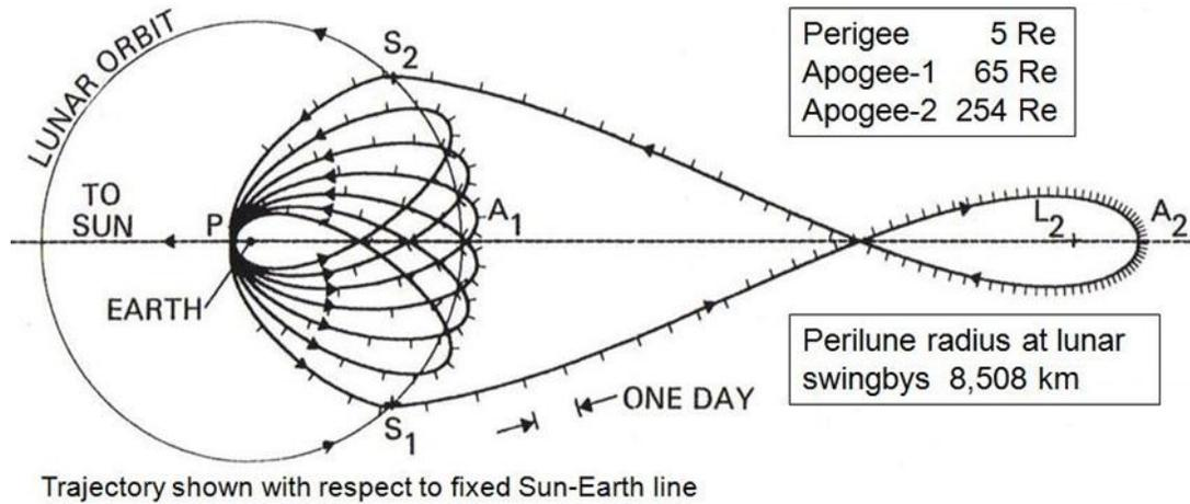
**Figure 13. Simplified Version of a Double Lunar-Swingby Trajectory (patched conic calculation).**
