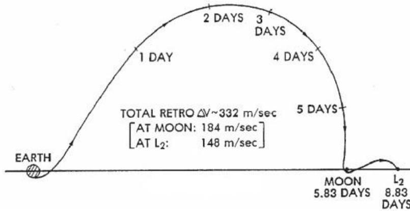
**Figure 2. Indirect transfer from a low-Earth parking orbit to the Earth-Moon L2 point. This is a rotating lunar orbit plane view with a fixed horizontal Earth-Moon line. [8, 10].**
