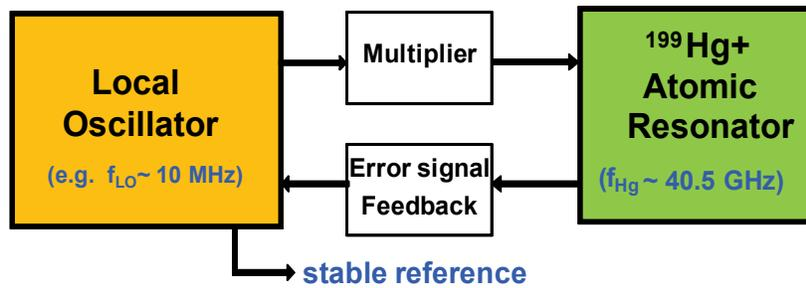
**Figure 5:** Mercury ion clock disciplining a Local Oscillator.
