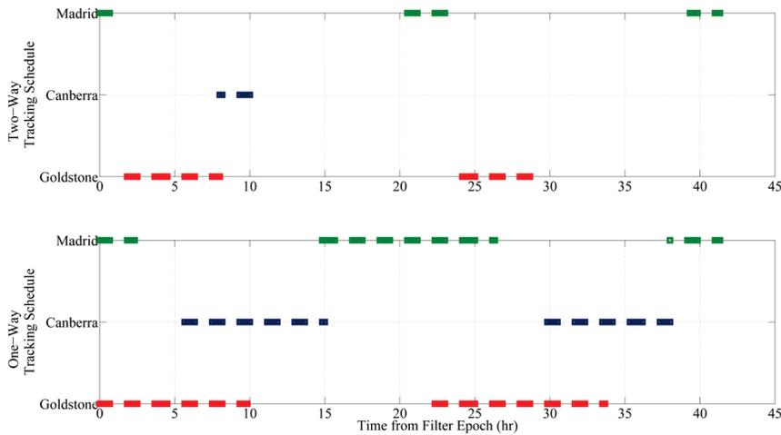
**Figure 1:** Simulated DSN tracking schedule for Mars orbiter example.
