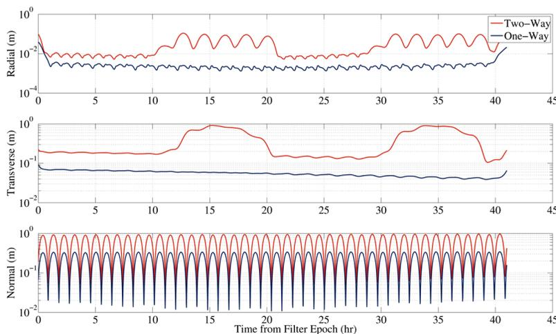
**Figure 2:** Comparison of estimated position uncertainty ( $1\sigma$ ) for 2-Way and 1-way Doppler tracking.
