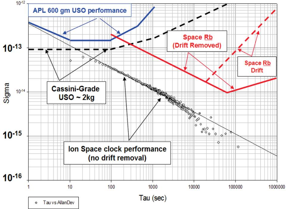
**Figure 7:** Measured (frequency domain) clock stability (Allan Deviation) of a sealed tube prototype  $^{199}\text{Hg}$  ion clock. A typical GPS Rubidium space clock (red) and USO (blue and black dash) is shown. The Ion Clock data shows no significant frequency drift.
