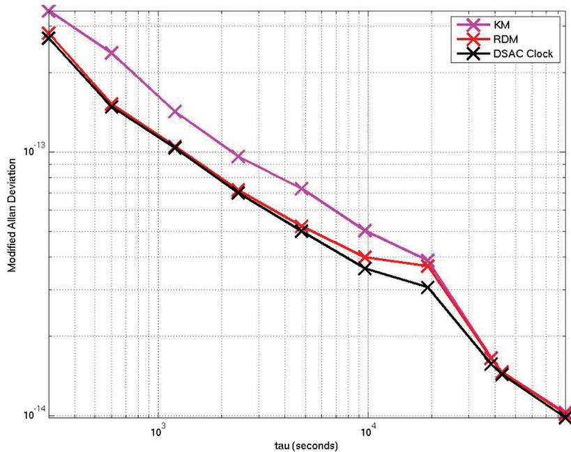
**Figure 9:** DSAC simulation result for a 600 km orbit. Plot of MAD versus  $\tau$  between 300 s and 1 day for KM (magenta), RDM (red), and input clock (black) with  $\sigma_y(1 \text{ day}) = 10^{-14}$  (project required clock performance). Note improvement of RDM over KM and that  $\sigma_y(1 \text{ day}) = 2 \times 10^{-14}$  (required clock validation) is easily met.
