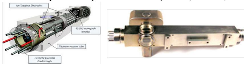
**Figure 6:** Ion trap/ vacuum tube assembly engineered following space vacuum tube design principles and bake-able to 450 C.
