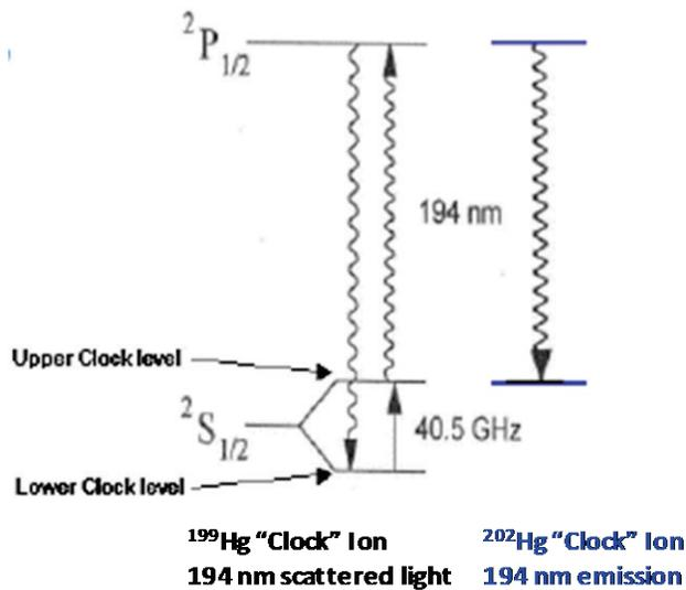
**Figure 4:** Mercury ion clock transition and UV transition for state selection/detection.
