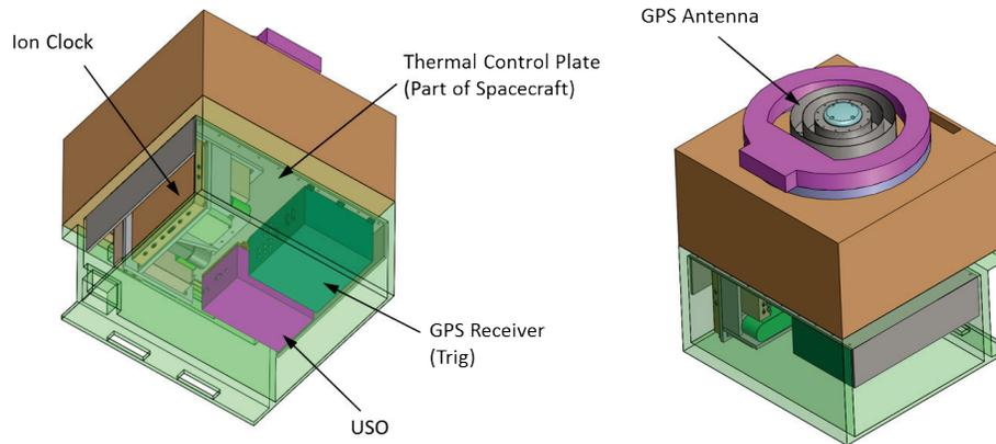
**Figure 8:** Candidate payload configuration on a LEO spacecraft.
