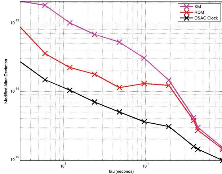
**Figure 10:** DSAC simulation result for a 600 km orbit. Plot of MAD versus  $\tau$  for KM (magenta), RDM (red), and the input clock (black) with  $\sigma_y(1 \text{ day}) = 10^{-15}$  (expected clock performance). Note large improvement of RDM over KM and that  $\sigma_y(1 \text{ day}) = 2 \times 10^{-14}$  project requirement is easily met.
