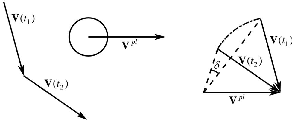
Fig. 2. Geometry of the gravity assist maneuver.
