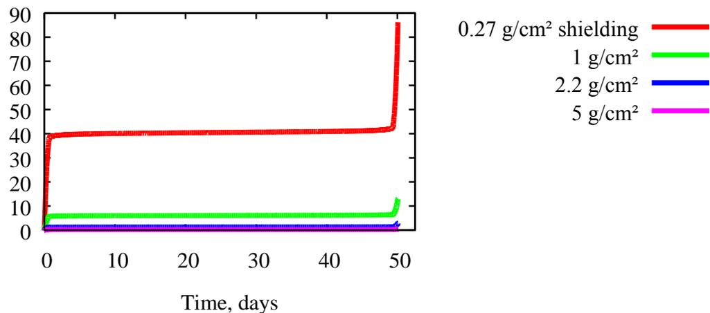
**Figure 7. Dynamics of radiation dose accumulation (TILD) in the vicinity of Jupiter in one orbital revolution for various protection levels (in  $\text{g}/\text{cm}^2$ ).**
