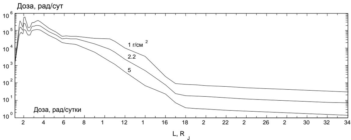
**Figure 6. Radiation level in the vicinity of Jupiter [40]; the distance from the center of Jupiter in terms of its radius is plotted on the horizontal axis.**
