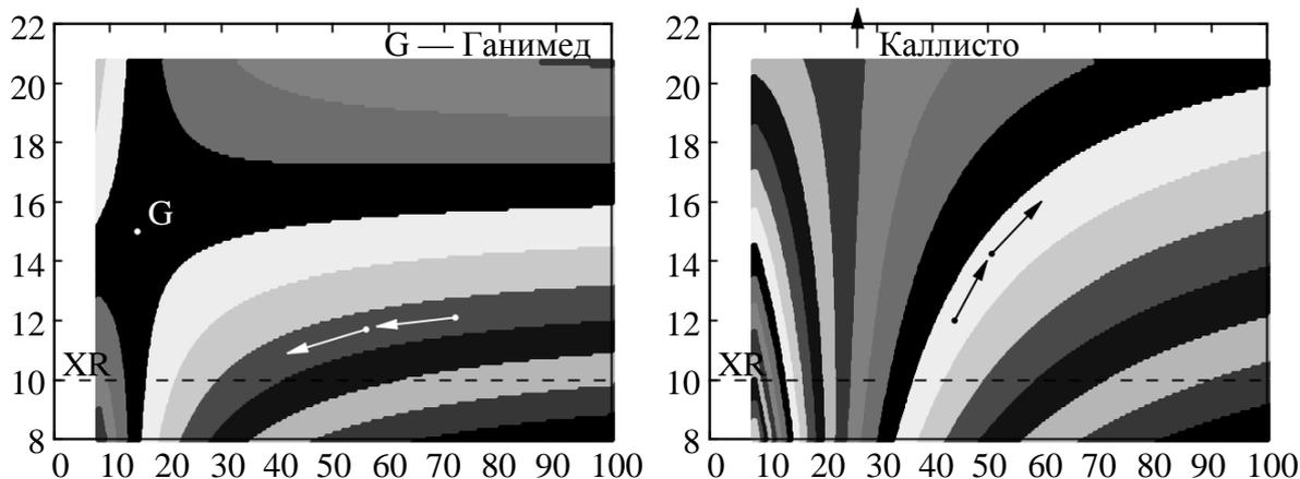
**Fig. 4. Isoinfines on Tisserand—Poincare diagrams for Ganymede and Callisto; the apocenter and pericenter altitudes are given in terms of the Jupiter radius  $R_J$ .**
