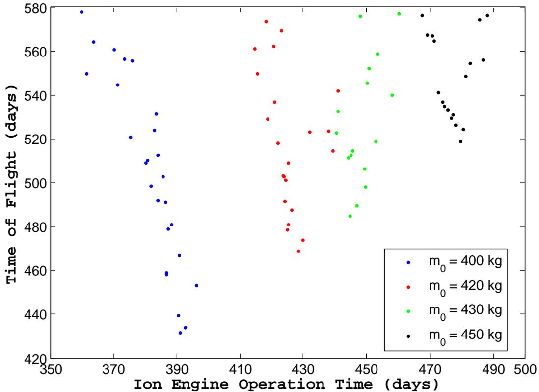
**Figure 3. Time of Flight vs Ion Engine Operation Time.**
