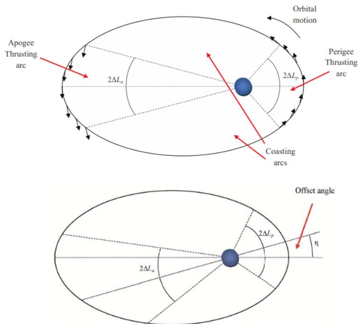
Figure 2. Simplified Low-Thrust Control Scheme: Symmetric (Top) and Asymmetric Thrust Pattern (Bottom).
