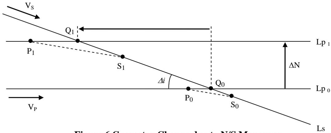
**Figure 6 Geometry Change due to N/S Maneuver**
