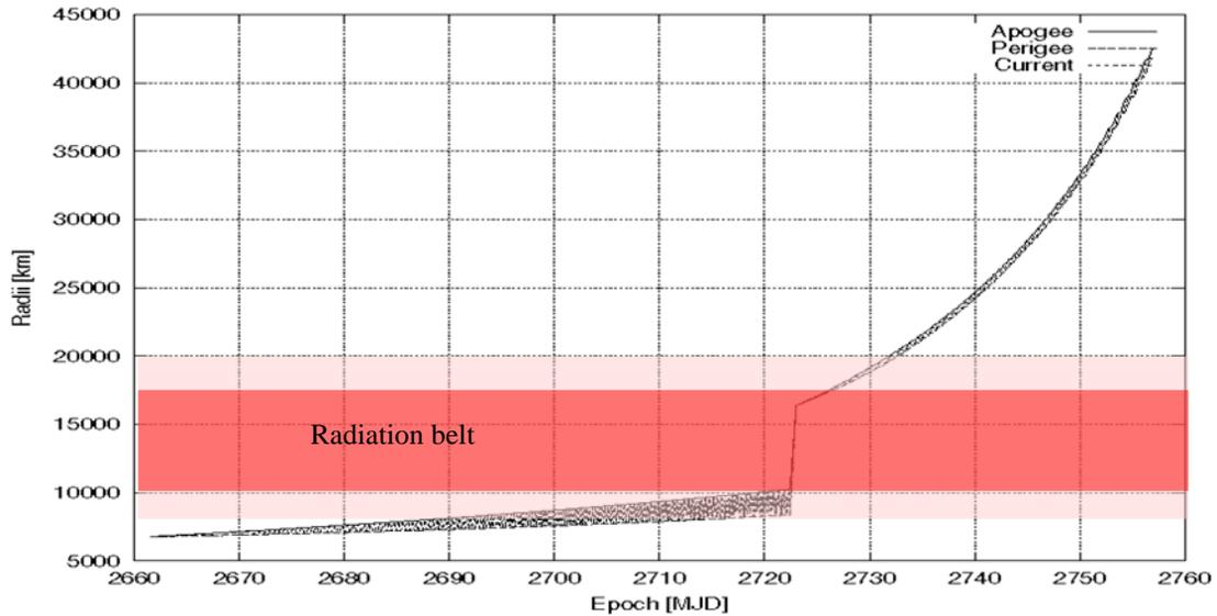
**Figure 2: Proposed E-Vega altitude profile for a solar-electric transfer from LEO to GEO including one chemical manoeuvre to skip the radiation belts [5].**
