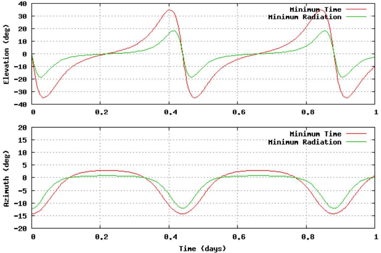
**Figure 8: Time history of elevation (= in-plane component, top panel) and azimuth (=out-of-plane component, bottom panel) of the thrust vector during the first two orbits of the two different transfers from GTO to GEO (t=0 is at apocentre, t=0.22 days is at pericentre after half an orbit).**
