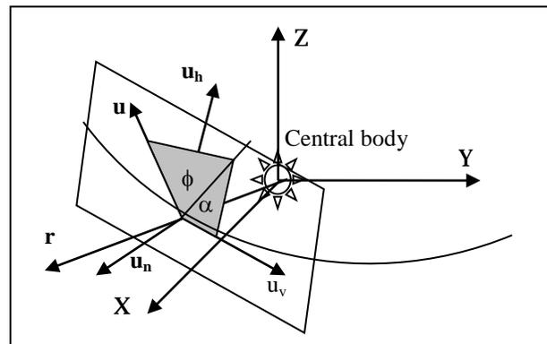
**Figure 1: Definition of thrust angles elevation  $\phi$  and azimuth  $\alpha$  in a local reference frame.**
