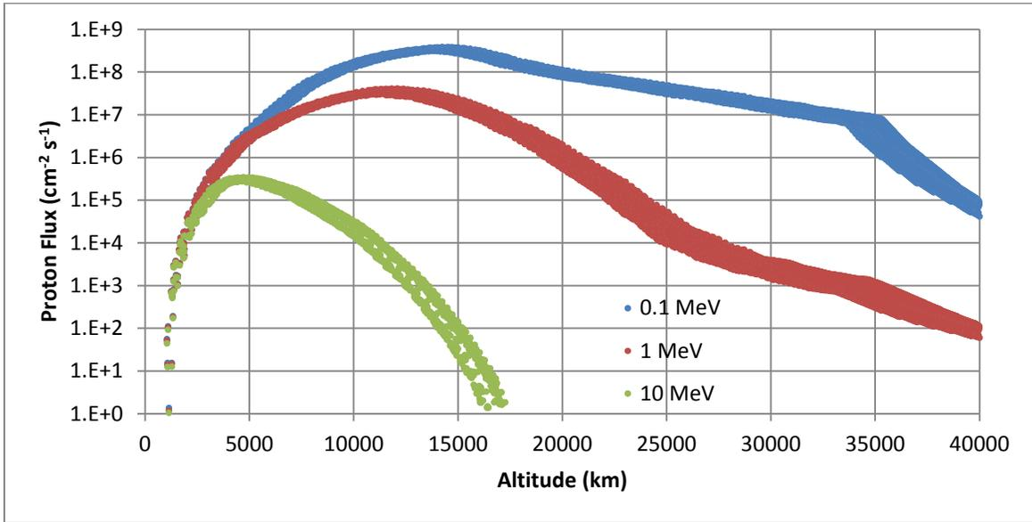
**Figure 3: Proton flux as function of altitude during a 172-day SEP transfer from GTO to GEO**
