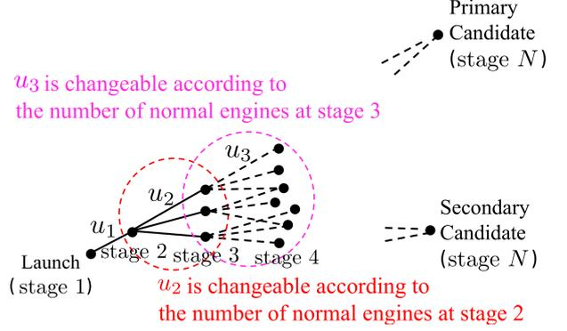
Fig. 2. Resulting trajectory branches according to the number of normal engines.
