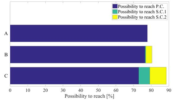
Fig. 5. Possibility to reach each candidate when defining the failure possibility as 2%. "A" indicates the fuel minimum solution to primary candidate aiming at only primary candidate, which is conventional method. "B" indicates the fuel minimum solution to primary candidate considering secondary candidates. "C" indicates that optimal solution in this simulation.
