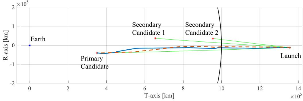
Fig. 3. Resulting trajectory of the simulation with 2% failure possibility. Observe that blue trajectory bends towards secondary candidates. Blue line and red dotted line mean the optimal trajectory in case of 2% failure possibility and 3% failure possibility, respectively.
