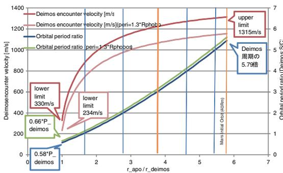
Fig. 5. Apoapsis altitude, orbital period and relative velocity in Deimos flyby.
