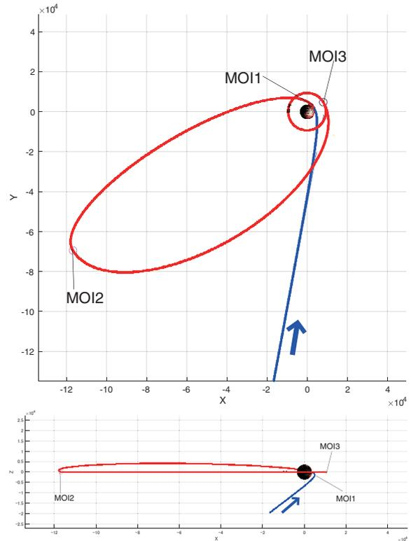
Fig. 4. Orbit diagram for MOI1-3.
