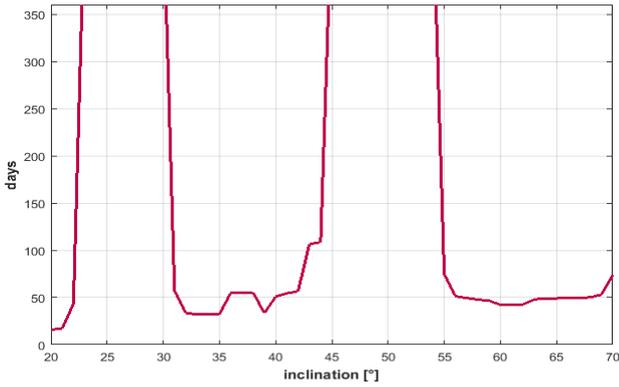
Fig. 3. Lunar mission lifetime profile in 100km altitude circular orbit.
