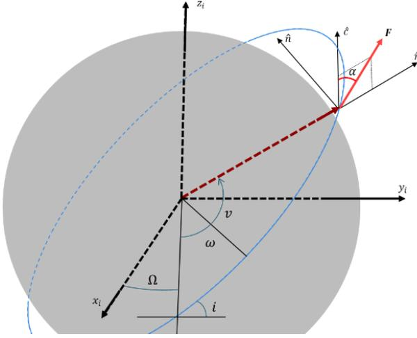
Fig. 6. Geometry of the reference frame used to compute the thrust direction  $F$ .
