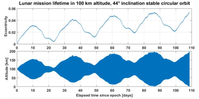
Fig. 5. Evolution of the eccentricity and lunar altitude within an unstable orbit.
