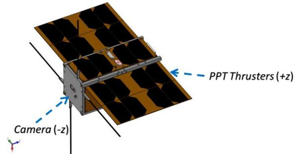
Fig. 1. Aoba VELOX-4 satellite 3D view.
