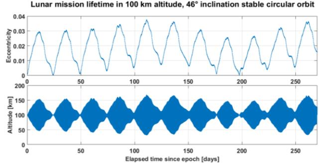
Fig. 4. Evolution of the eccentricity and lunar altitude within a stable orbit.
