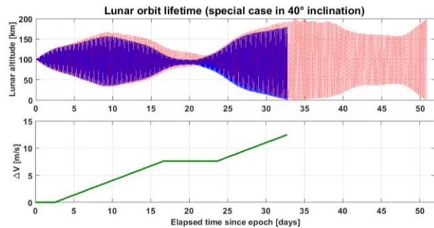
Fig. 10. Special case when lifetime reduction resulted by implementing the proposed orbit control strategy.
