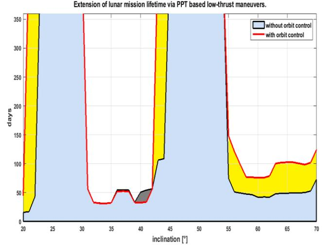
Fig. 7. Simulation results considering a range of initial inclinations for a lunar orbit mission and the extension of the mission lifetime.
