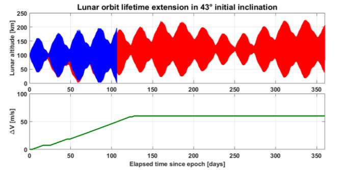
Fig. 8. Mission lifetime extension profile by considering a  $43^\circ$  initial inclination.
