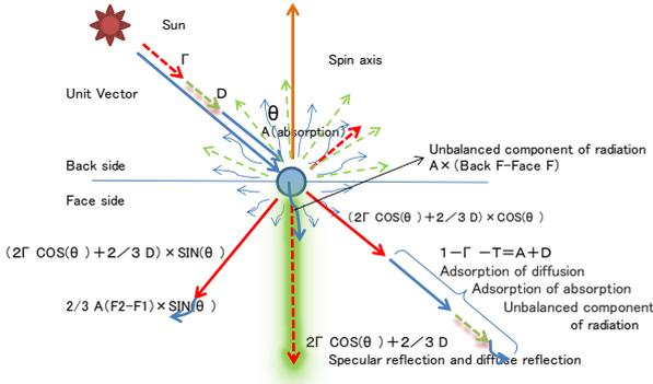
Fig. 3.1 Conceptual diagram of solar radiation pressure model of IKAROS
