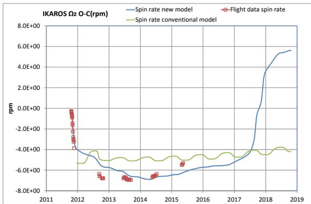
Fig. 6.1 Spin rate by observation data and motion model
