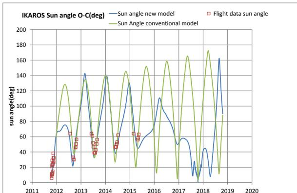
Fig. 6.2 Sun angle by observation data and motion model
