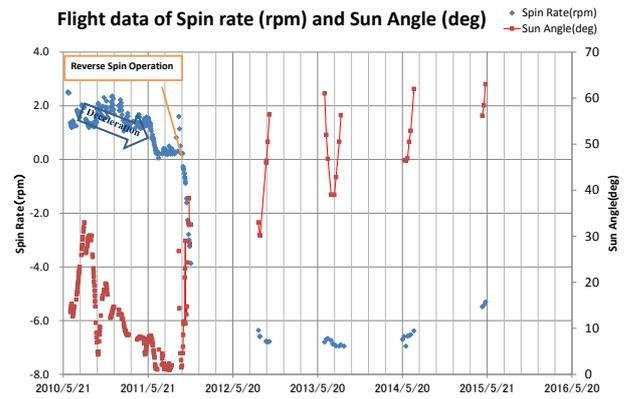
Fig. 3.3 Flights data of spin rate and sun angle
