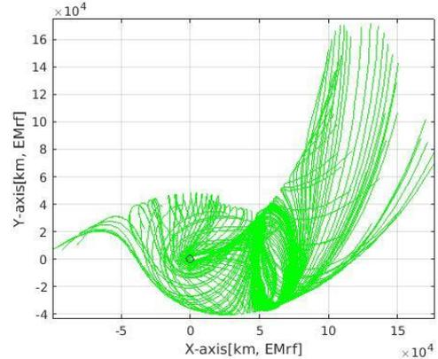
Fig. 7. Trajectories propagated backward in time by applying small velocity perturbation to minimum stretching directions from a quasi-periodic halo orbit around lunar L<sub>2</sub> in the Moon-centered Earth-Moon rotating frame.
