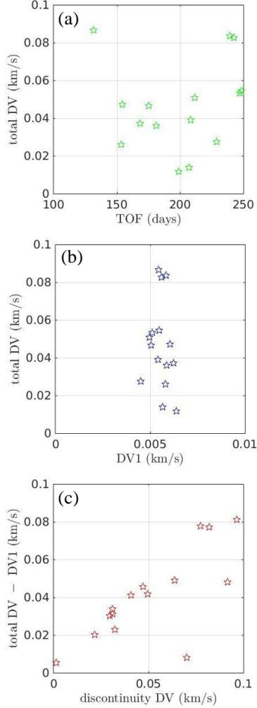
Fig. 10. (a) TOF and total  $\Delta v$  of optimal solutions. (b)  $\Delta v_1$  and total  $\Delta v$  of optimal solutions. (c) Discontinuity  $\Delta v$  of the initial guesses and  $\Delta v$  subtracting  $\Delta v_1$  from total  $\Delta v$  after optimization.
