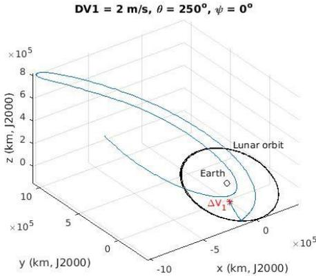
Fig. 5. An example of a trajectory propagated forward in time with  $\Delta v_1=2$  [m/s] in the Earth-centered J2000 frame.
