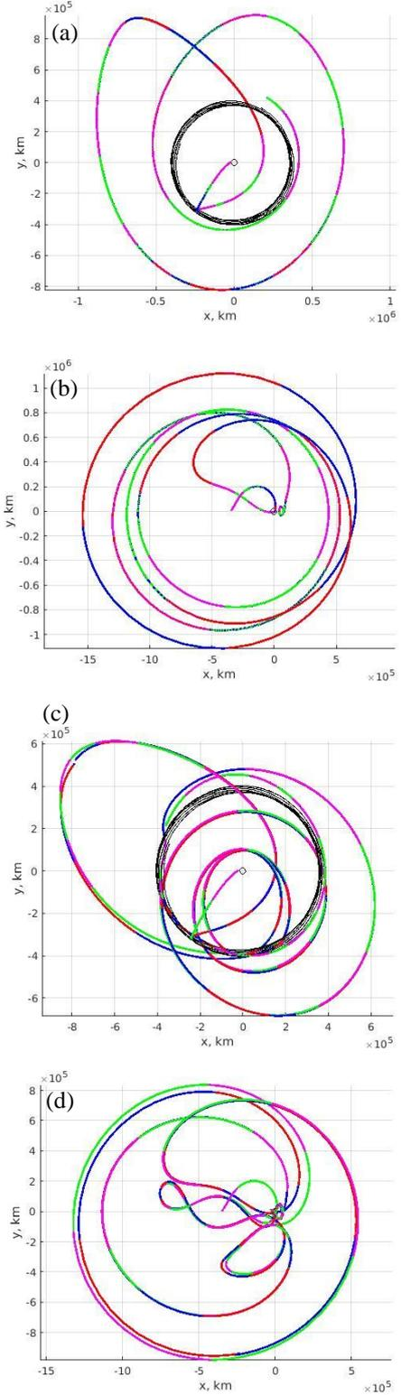
Fig. 11. Optimal transfer trajectories with (a), (b) total  $\Delta v=11.5$  [m/s],  $\Delta v_1=6.4$  [m/s], TOF=199 [days], and (c), (d) total  $\Delta v=13.7$  [m/s],  $\Delta v_1=5.7$  [m/s], TOF=207 [days] in the (a), (c) Sun-Earth and (b), (d) Earth-Moon rotating frames, respectively. The red and blue arcs represent the initial guess, and the green and magenta arcs represent the optimal solution.
