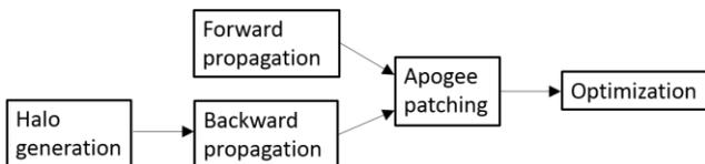
Fig. 3. A flowchart of the trajectory design approach for EQUULEUS.
