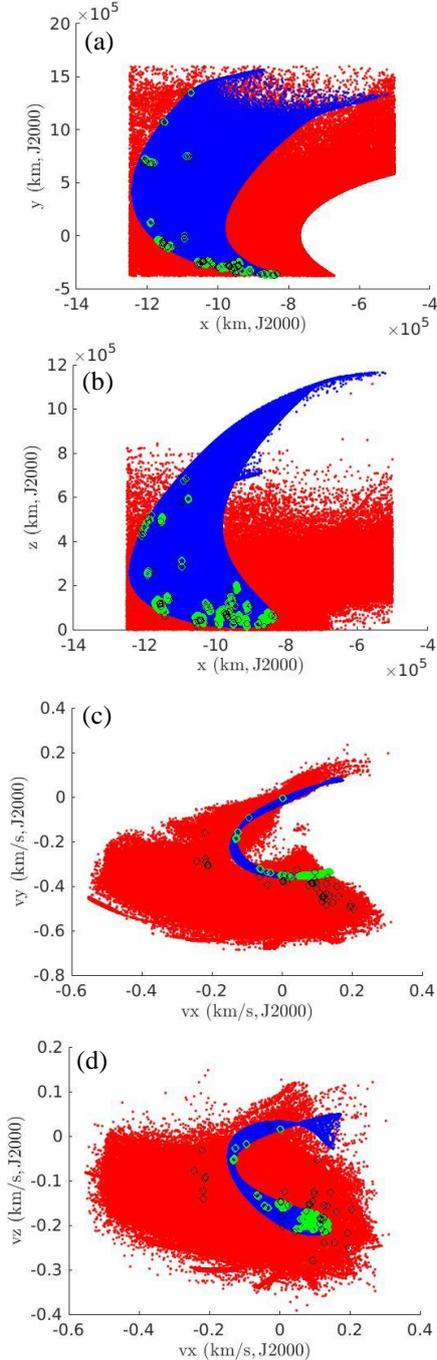
Fig. 8. Forward ( $\Delta v_1=6$  [m/s], blue) and backward (red) states at apogees, displayed with those satisfying the tolerances  $\text{TOLE.t}=0.025$ [days] and  $\text{TOLE.rmag}=25,000$ [km] (green for forward and black for backward) in (a) x-y, (b) x-z, (c) vx-vy, (d) vx-vz planes in the Earth-centered J2000 frame.
