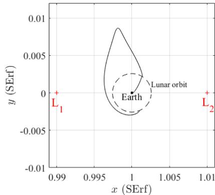
Fig. 2. An example of low-energy transfer to the Moon computed in Oshima et al.<sup>16)</sup> The trajectory is shown in the non-dimensional Sun-Earth rotating frame.
