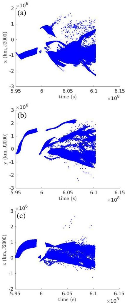
Fig. 6. (a) x, (b) y, (c) z at apogees of trajectories propagated forward in time in the Earth-centered J2000 frame in terms of ephemeris time.
