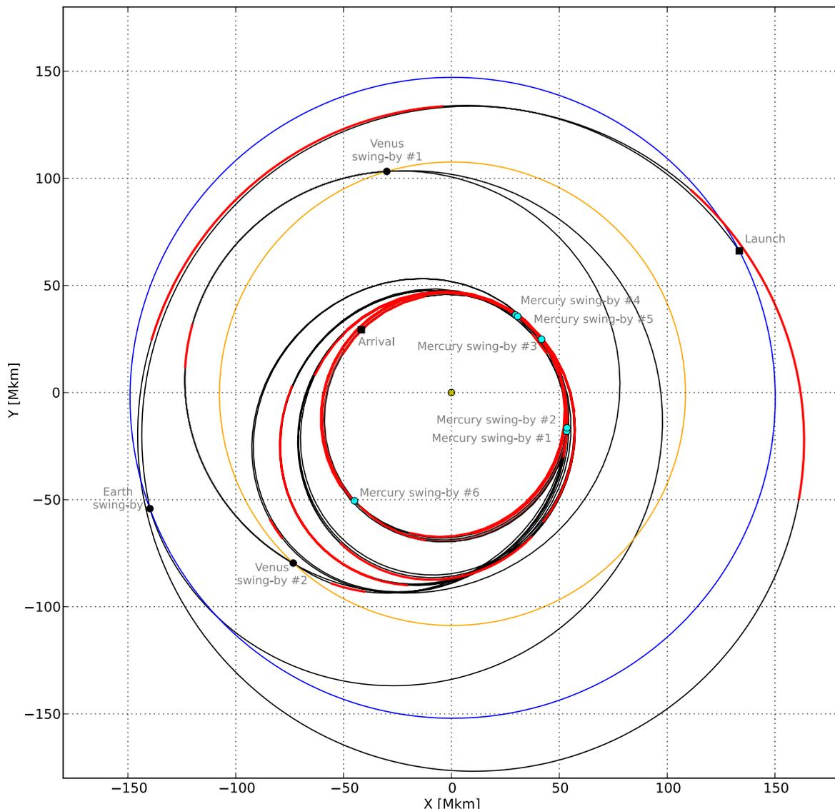
Fig. 3: BepiColombo cruise trajectory projected in the ecliptic plane
