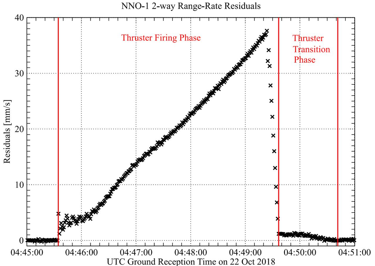
Fig. 8: A-priori Doppler residuals (count time of 1s) for the axial test OCM, pass-through against orbit with predicted manoeuvre acceleration profile.
