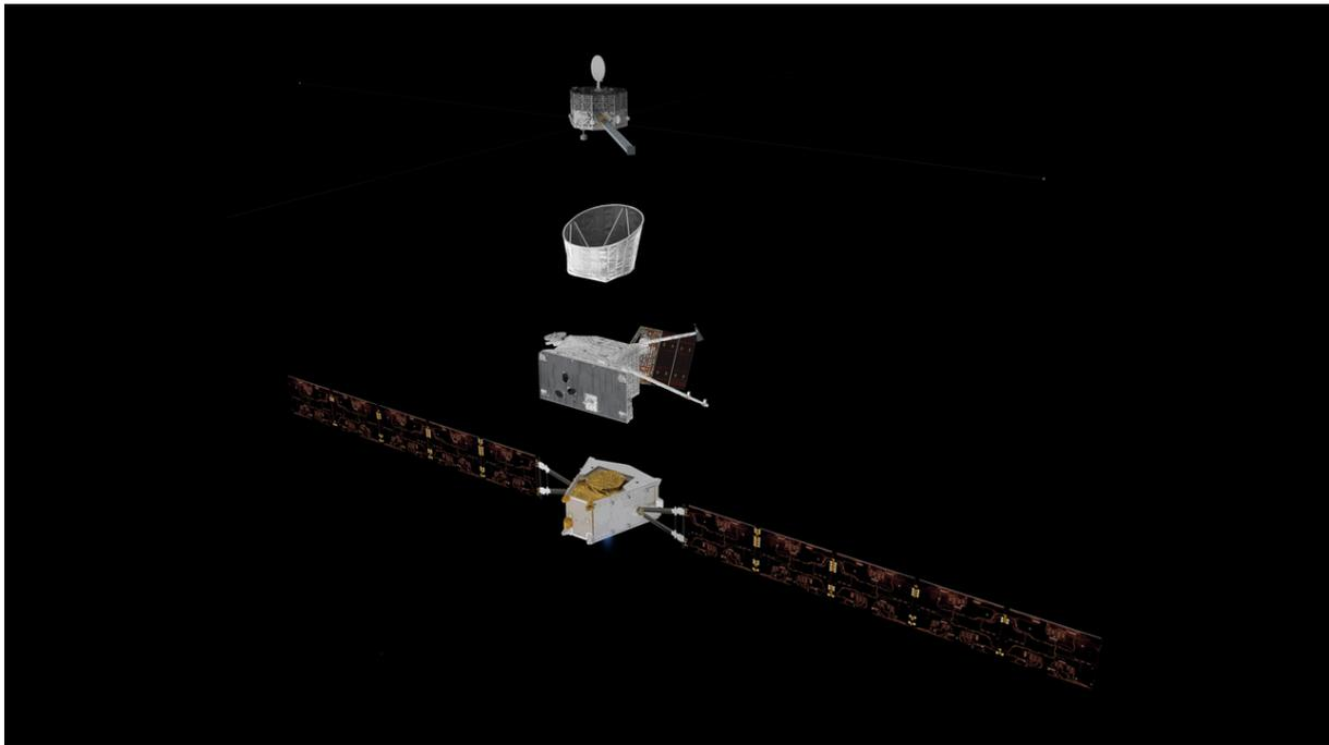
*Fig. 1: BepiColombo spacecraft stack in exploded view*
