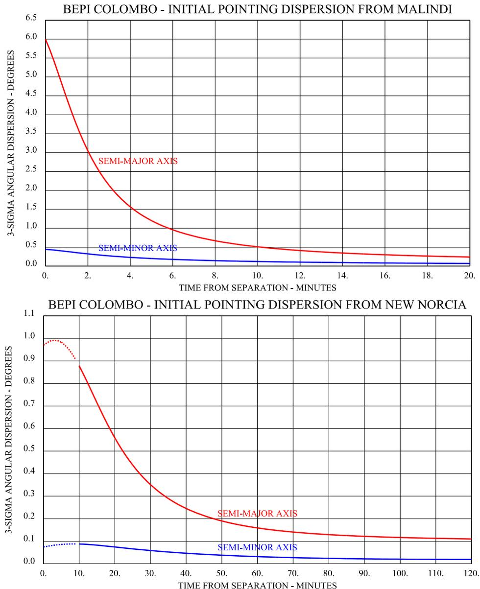
Fig. 5: Initial pointing dispersions from New Norcia (top) and Malindi (bottom)
