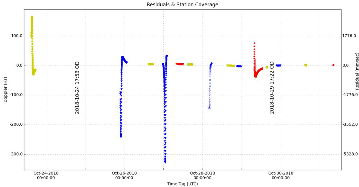
Fig. 6: Ground Doppler frequency prediction performance during a week in XMO7
