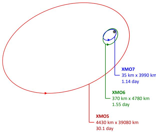
XMO7 was the final orbit for Dawn's mission. The main goal of XMO7 was to reach a low enough altitude to significantly improve the resolution and sensitivity of GRaND's nuclear spectroscopy data. There were several issues and factors that were considered in the design of XMO7, including orbit stability for planetary protection, efficient usage of the remaining hydrazine stores, and the targeting of a peridemeter pass over a specific Ceres surface feature (Cerealia Facula in Occator crater).
