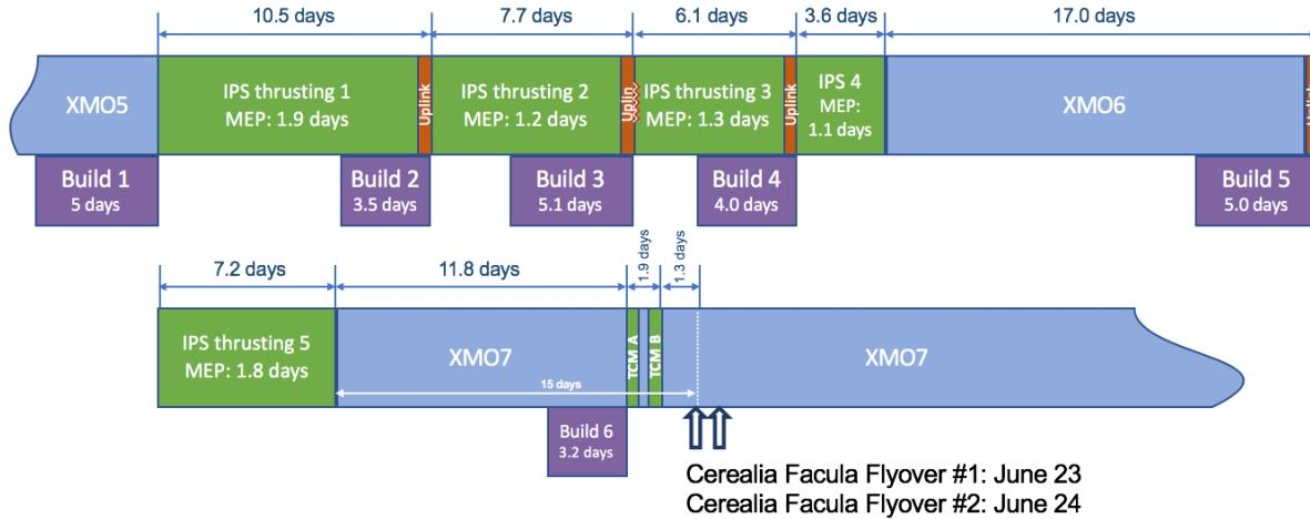
Fig. 4: Transfer architecture from XMO5 to XMO7. The maneuver expansion period (MEP) is an allocation of additional time for statistical IPS thrusting
