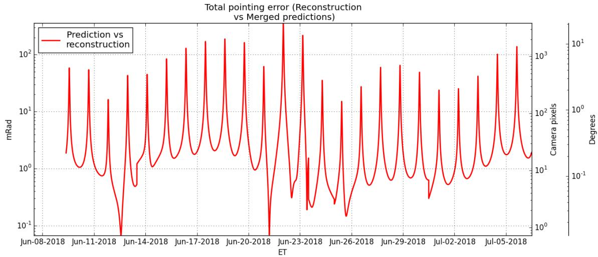
Fig. 7: Pointing prediction performance during first part of XMO7
