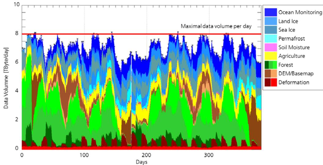
Fig. 3: Data volume of an exemplary timeline for the Close Formation for one year.
