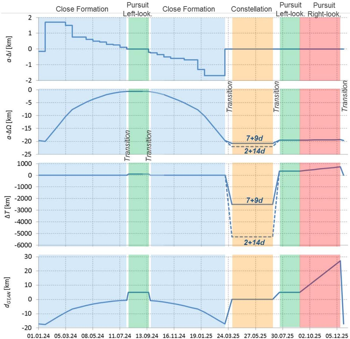
Fig. 4: Evolution of optimized formation parameters within a repeating two-year mission cycle. A constant vertical separation of 600 m applies to all Close Formation phases. Two options are depicted for the constellation phase, i.e. 7+9d and 2+14d constellations.
