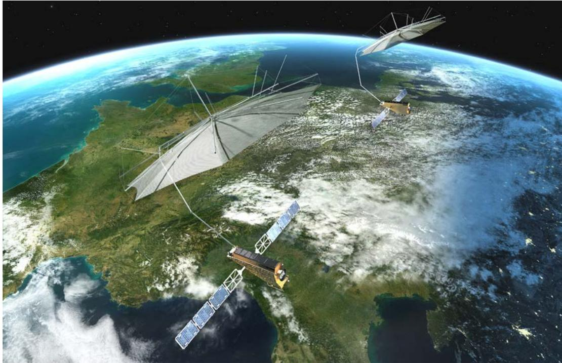
*Fig. 1: Artistic view of the Tandem-L formation in 741 km altitude. Each spacecraft weighs about 3 tons and carries a deployable reflector antenna with a diameter of 15 m.*
