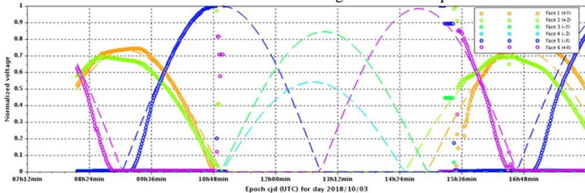
Fig. 8 Comparison between the PEC observed voltages (colour circles) and the predicted voltages (dashed lines) based on the attitude determination. The absence of observed voltages is due to asteroid night.
