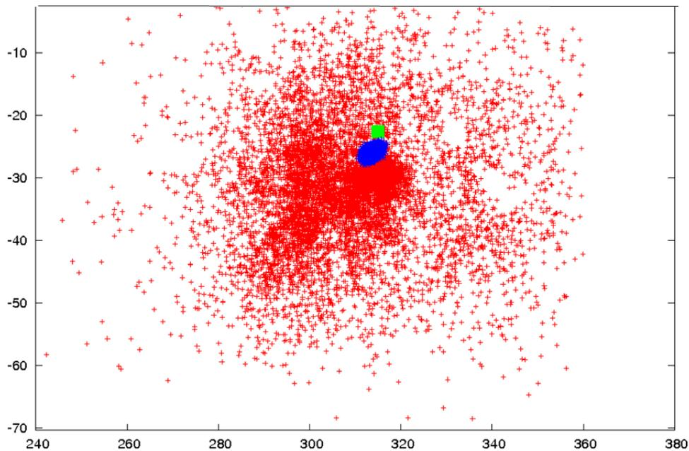
*Fig. 7 Trajectories predictions based on the first assessment of Hayabusa2 position and velocity at MASCOT's release provided by JAXA. In blue: simulated locations of MASCOT's first contact with the surface. In red: simulated locations of MASCOT's first rest point (taking into account bounces). In green: actual position of the first contact point, voluntarily enlarged to be visible.*
