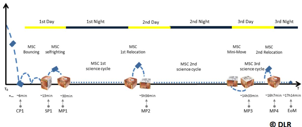
*Fig. 1 Illustration of the main stages of MASCOT's mission. CP1 stands for first contact point, SPi for ith Settlement Point, MPi for ith Measurement Point (location after uprighting), EoM for End of Mission*
