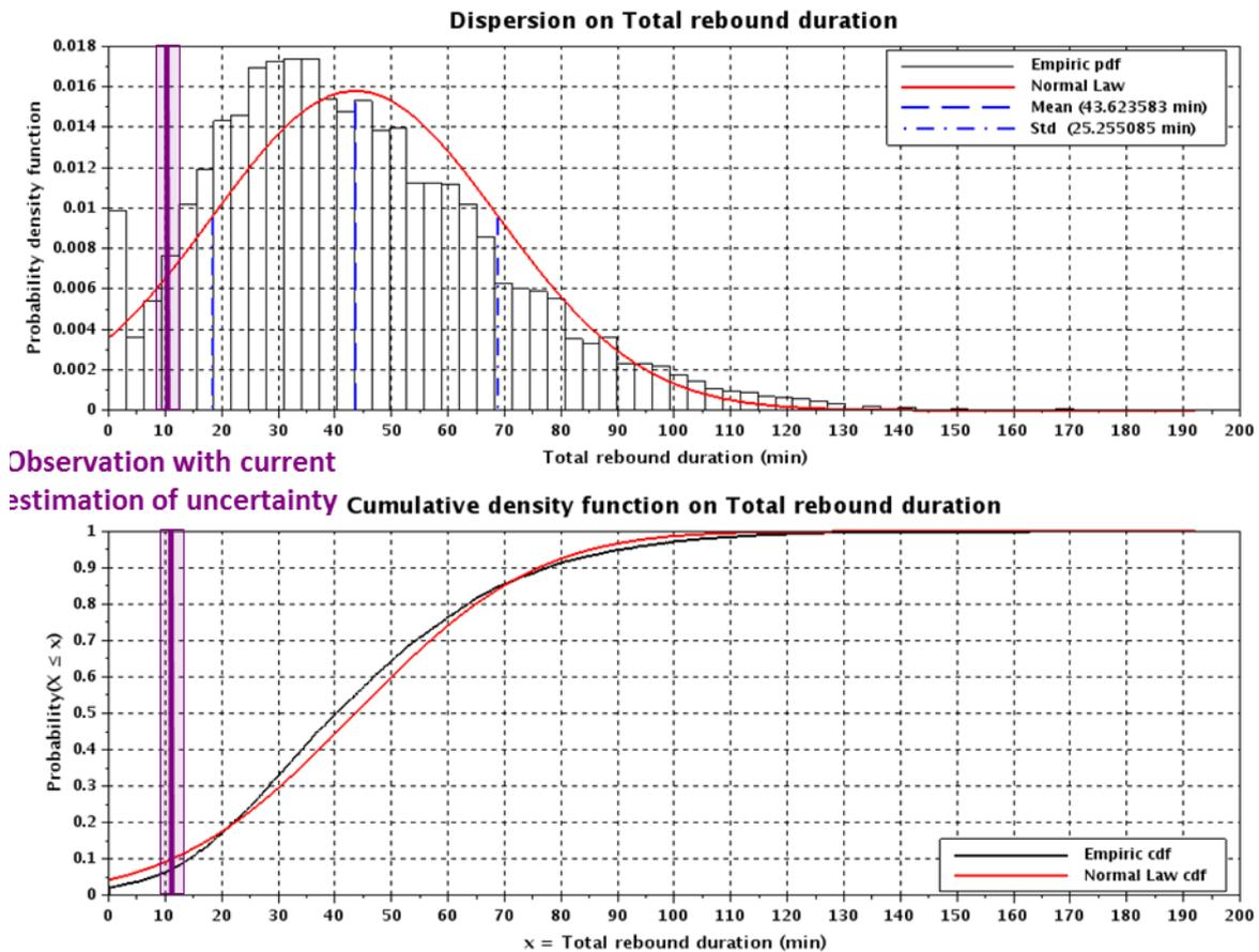
Fig. 5 Probability density and cumulative density function for total rebounds duration (time between the first contact on the asteroid and the first rest point after rebounds) computed from Monte-Carlo simulations before landing.
