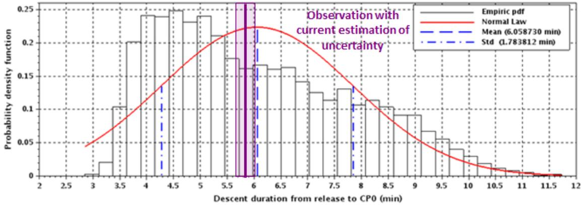
Fig. 4 Probability density for descent duration (CP0 = first contact point on asteroid’s surface) computed from Monte-Carlo simulations before landing.
