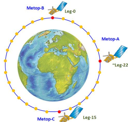
Fig. 12: Metop-A/B/C nominal Trident configuration
