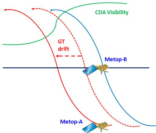
Fig. 13: Impact of ground-track drift on ANX to AOS time
