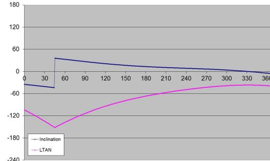
*Fig. 6: Expected Metop-C LTDN deviation after launch for large negative injection error plus correction at extended window limit*
