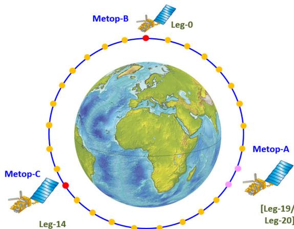
Fig. 15: Metop-A/B/C Tristar configuration
