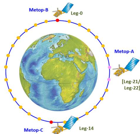
Fig. 14: Metop-A/B/C alternative Trident configuration
