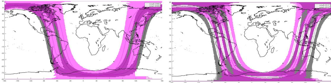
Fig. 16: Coverage figure for Metop-B/C Trident configuration (GOME, ASCAT)
