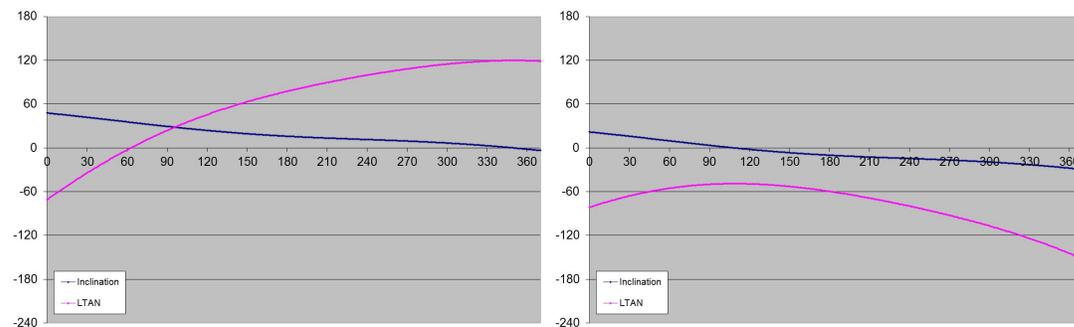
*Fig. 8: Expected Metop-C LTDN deviation after launch for moderate injection error cases*
