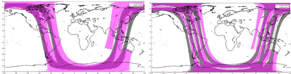
Fig. 17: Coverage figure for Metop-B/C Tristar configuration (GOME, ASCAT)
