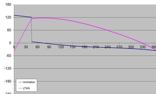
*Fig. 7: Expected Metop-C LTDN deviation after launch for large positive injection error plus correction at nominal window limit*
