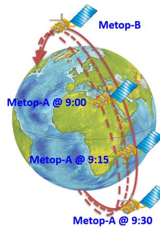
Fig. 3: Metop-A relative phase evolution with LTDN drift
