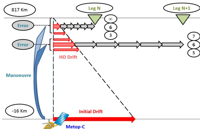
Fig. 11: Metop-C acquisition on first target
