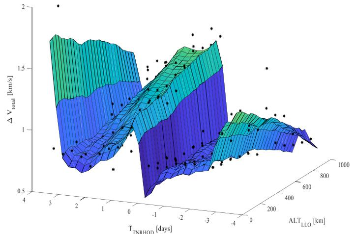
Fig. 3: MDO data points and surrogate prediction for  $\Delta V_{total}$
