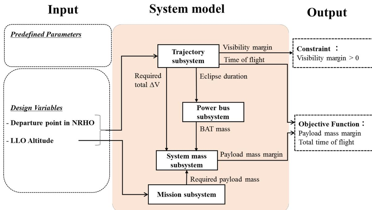
Fig. 2: MSDO system block diagram
