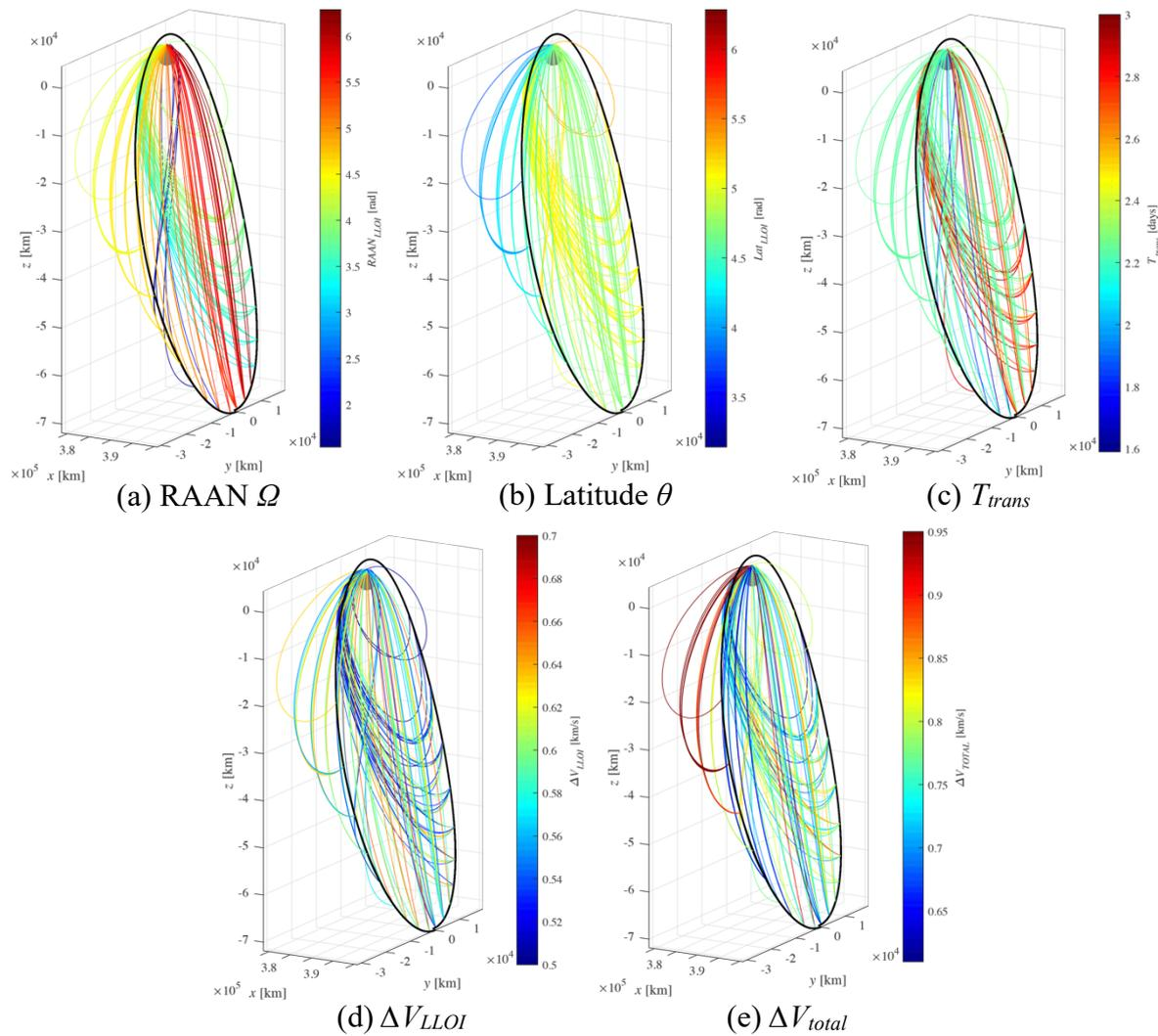
Fig. 5: Feasible transfer trajectories from MDO (converged with *fmincon*)
