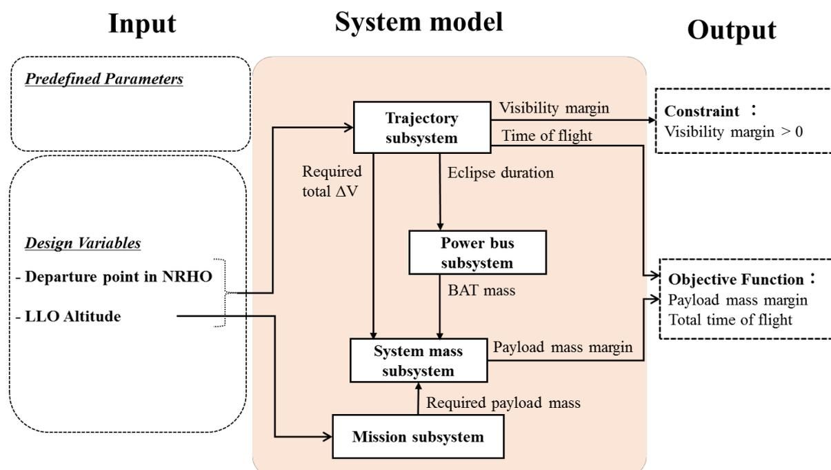
Fig. 2: MSDO system block diagram
