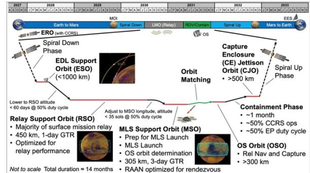
Figure 13: ERO Mission in Low Mars Orbit
