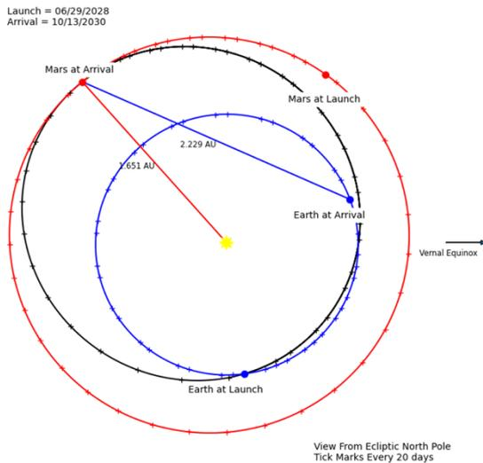
Figure 6: SRL Cruise Trajectory for the Open of the Launch Period
