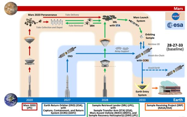
Figure 1: Mars Sample Return Architecture as of 2023
