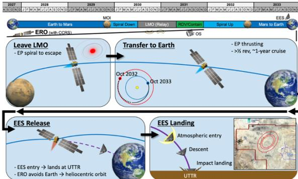
Figure 14: ERO Mission from Low Mars Orbit to Earth Return
