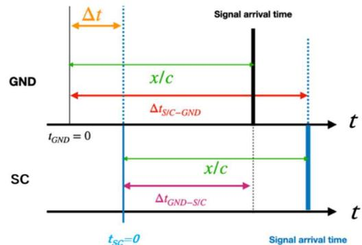
Fig. 2. Conceptual Drawing of the Signal Flow in Asynchronous One-Way Ranging Scheme
