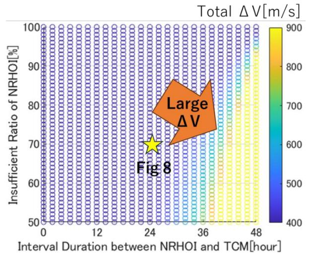
Fig. 9. Relationship between Insufficient NRHOI, Interval Duration of TCM, and  $\Delta V$
