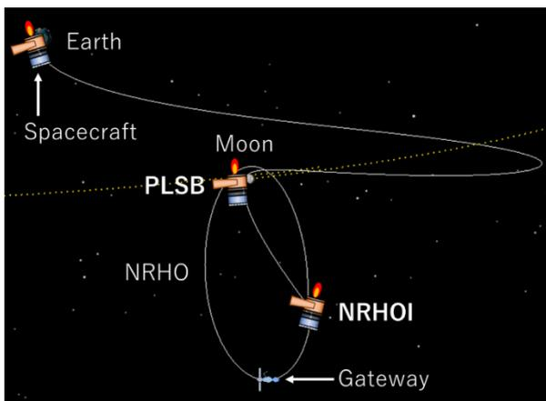
Fig. 2. Trajectory of In-Direct Transfer (IDT)
