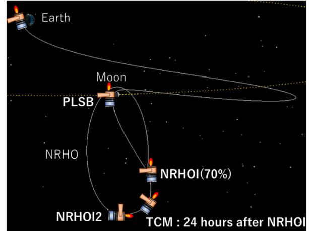
Fig. 8. Example of Recovery Trajectory in case of 70% NRHOI and TCM after 24 hours
