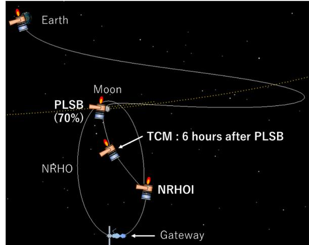
Fig. 4. Example of Recovery Trajectory in case of 70% PLSB and TCM after 6 hours
