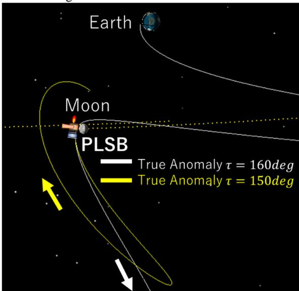
Fig. 12. Propagating trajectories of true anomaly = 160 and 150 degree after PLSB
