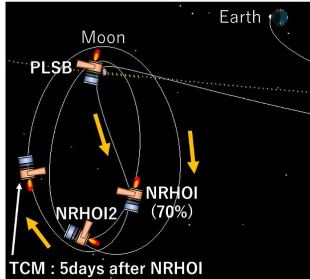
Fig. 10. Example of Recovery Trajectory in case of 70% NRHOI and TCM after 120 hours
