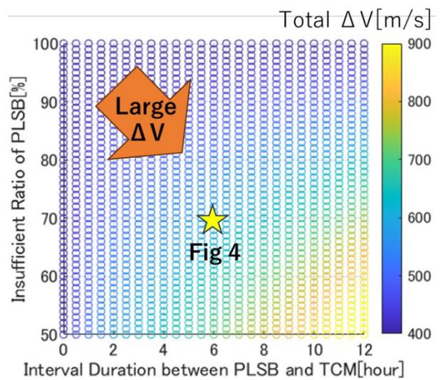
Fig. 5. Relationship between Insufficient PLSB, Interval Duration of TCM, and  $\Delta V$
