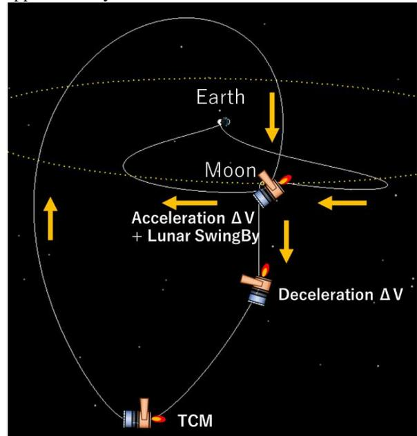
Fig. 7. Recovery trajectory in case of PLSB failure
