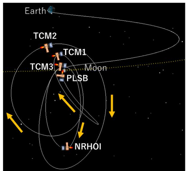
Fig. 14. Recovery trajectory in case of NRHOI failure
