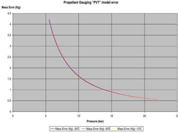
Fig. 3 Estimation of the propellant gauging error for the PVT model (Source: FOM)
