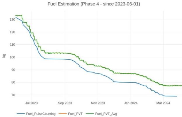
Fig. 7 S1B fuel estimation since the beginning of the deorbiting operations
