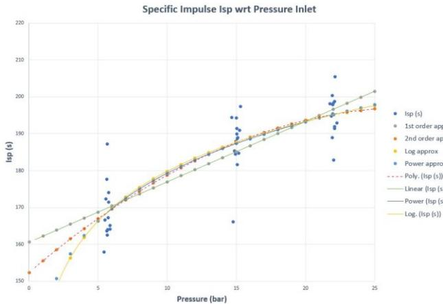
Fig. 4 Specific impulse characterisation wrt pressure input
