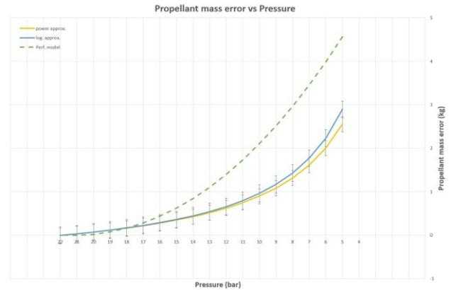
Fig. 5 Evolution of the propellant mass error for the power and the logarithmic models (PCM method)
