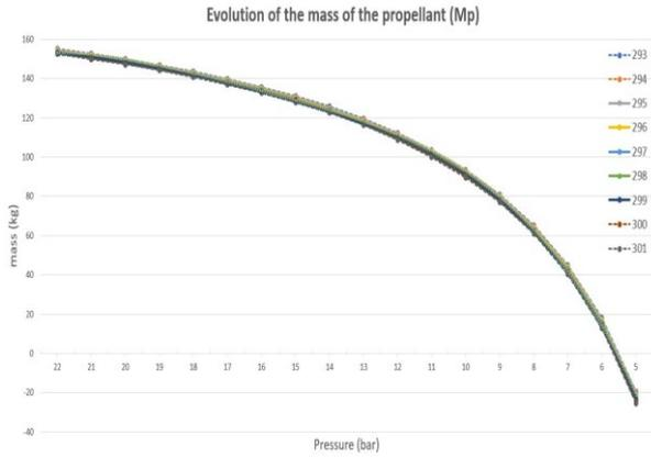
Fig. 1 Propellant mass prediction for different temperatures (in K)
