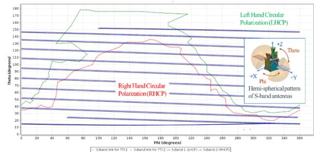
Fig. 2. On-board S-band antenna regions in Spacecraft Reference Frame together with the evolution (12 h) of the direction towards S-band ground stations in SAM.
