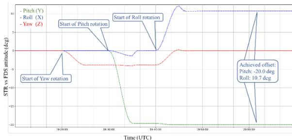
Fig. 13. FD monitoring of the attitude offset between the STR joined solution received in TM and the ground modelled unbiased FPM attitude during the attitude manoeuvre on 2023/07/20.
