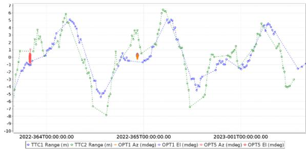
Fig. 4. S-band ranging and Optical measurements residuals after a 3-day alternate ranging campaign.
