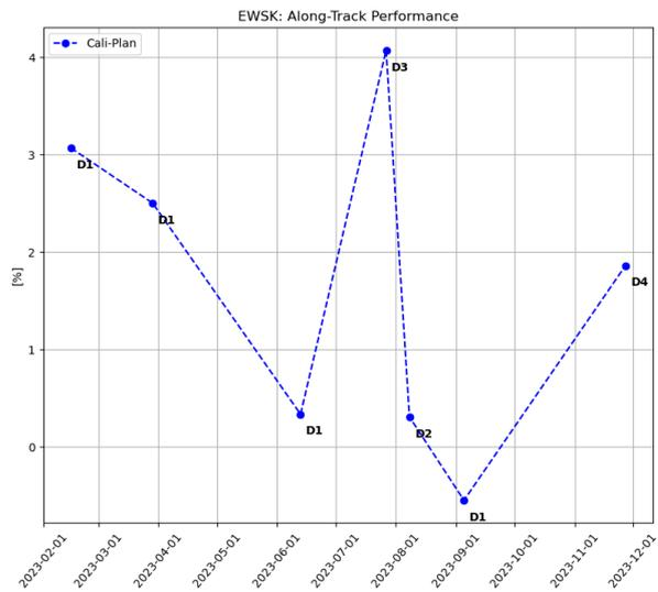
Fig. 10. Evolution of EWSK manoeuvre performance factors (LORF along-track component) for thrusters D.
