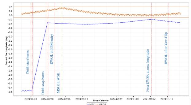
Fig. 16. Longitude evolution of MTG-I1 and MSG3 since the start of the MTG-I1 relocation campaign.
