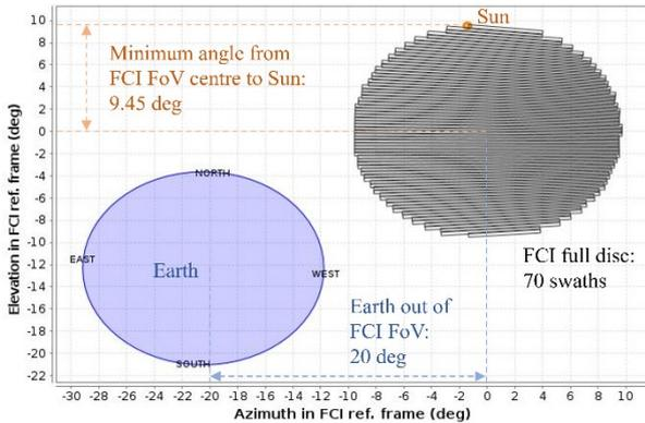
Fig. 12. FCI Sun straylight characterization test geometry in Yaw Flip Summer configuration, represented in FCI reference frame. Note the East/West direction inversion.
