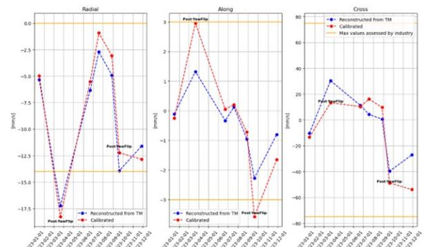
Fig. 7. Determined RWOL Delta-v in LORF components. Yellow lines show the maximum expected values.
