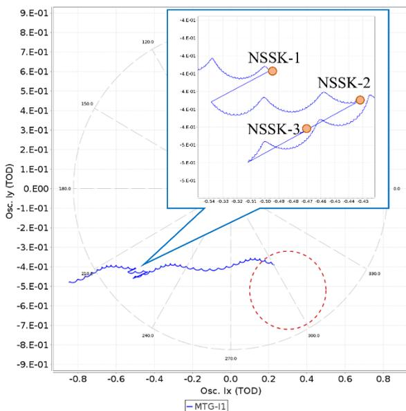
Fig. 11. TOD Inclination vector evolution from Hand-over, showing the effect of the NSSK test manoeuvres. The red circle is the control region for Routine Phase.
