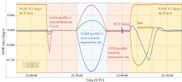
Fig. 15. GYR rates monitoring during drift-start burn-1 on 2024/01/23. Guidance attitude segments and SAM highlighted in different colours.
