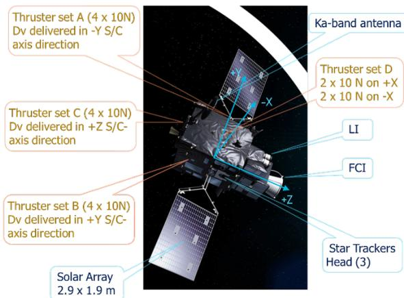
Fig. 1. MTG-I1 artistic impression depicting the S/C in FPM Summer season, together with a representation of the S/C reference frame.
