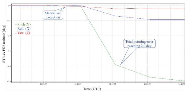
Fig. 8. Comparison of attitude quaternion produced by STR joined solution on-board and on-ground modelled attitude after EWSK manoeuvre on 2023/01/31.
