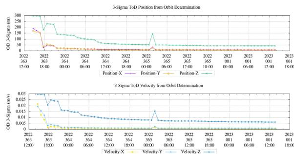
Fig. 3. Evolution of the determined position and velocity 3-sigma values during the 3 days alternate ranging campaign after Hand-over.
