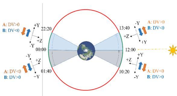
Fig. 14. Sun illumination constraints on S/C Y-axis for OTM using backup thrusters set (A/B). Manoeuvres can only be executed on the green orbit arcs.
