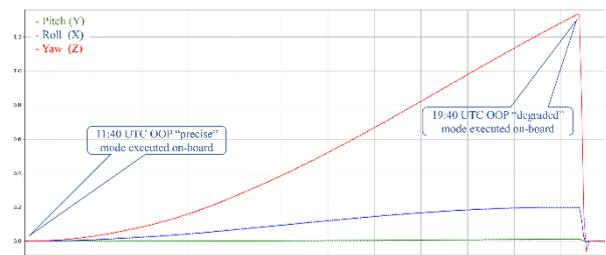
Fig. 6. Comparison of attitude quaternion produced by OOP function on-board and on-ground modelled attitude after the first OOP “precise” update.
