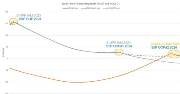
Fig. 8 Estimated LTAN evolution for the hybrid solution for the LTAN correction of Sentinel-5P wrt NOAA-2121, based on the propagation of the different orbits using the high precision propagator of NAPEOS
